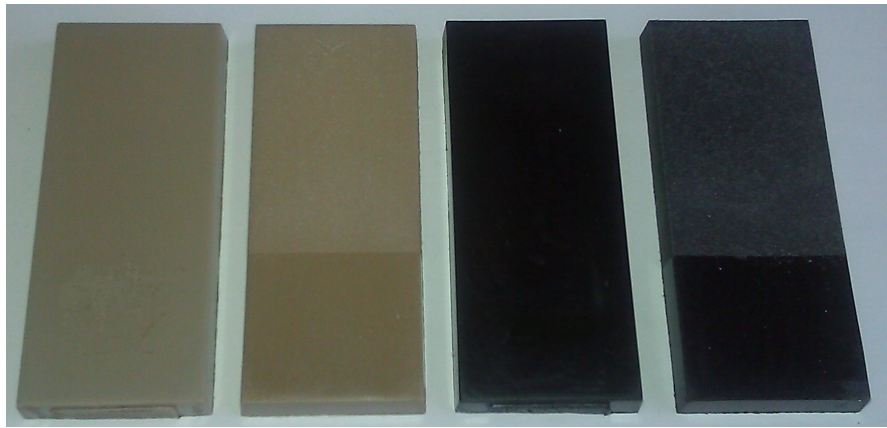
Figure 3.1: An example of each test plate used - From right to left: PEEK smooth injection moulded and grit-blasted finishes, and CFR-PEEK injection moulded and grit-blasted surface finishes
