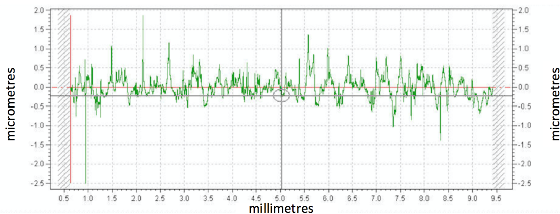
Figure 3.9: Roughness line profile on smooth injection moulded CFR-PEEK, with height in \mu\text{m} and length in mm
