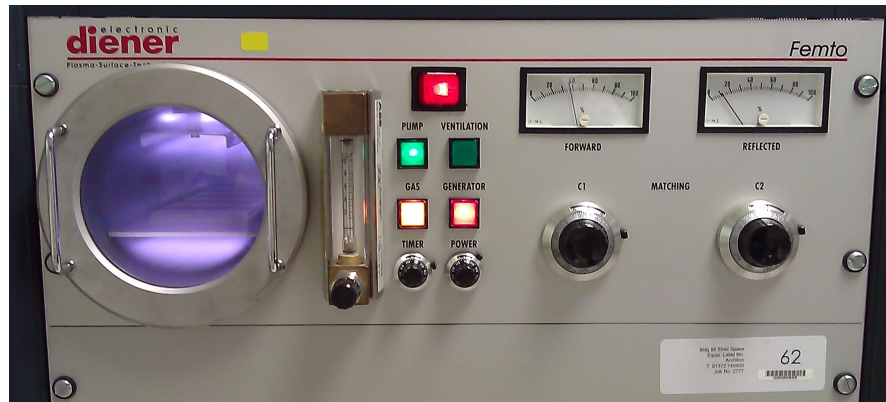
Figure 3.36: Plasma treatment of PEEK plates using a Diener Femto low pressure plasma system
