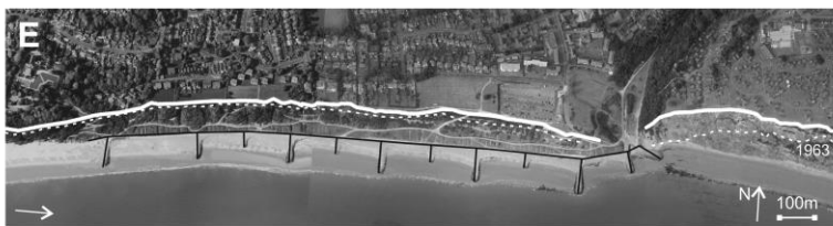
Set-back from 1.4km of groynes, seawalls, drainage and beach replenishment after the late 1960s.
