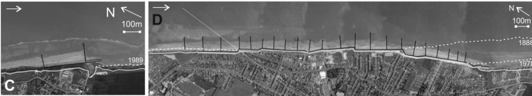
Set-back after 450m of rock armouring and groynes constructed in 1991.
