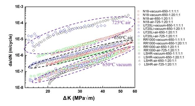
Fig. 1 Fatigue crack propagation rates in 4 advanced turbine disc superalloys  $^{5, 9, 21, 22}$ , where the figure legend indicates: alloy-environment-test temperature (in °C) - loading waveform (where 1:x:1:1 indicates a trapezoidal waveform: 1s ramp up, x s at maximum load, 1s ramp down and 1s at minimum load).
