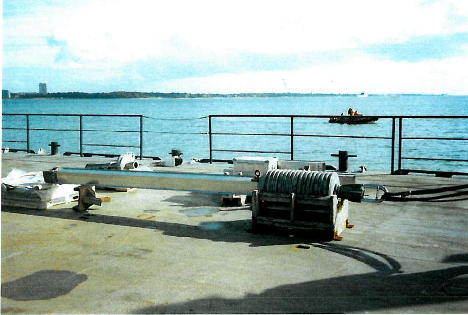
Figure 6.1. The Kastenlot core on deck before deployment.
