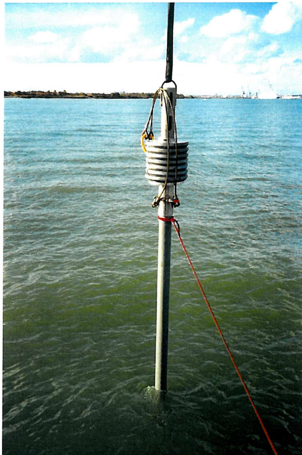
Figure 6.2. Deployment of the pressurised coring system.
