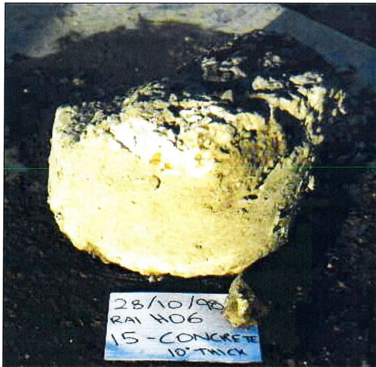
Figure 3.23 A 250mm thick piece of concrete recovered from H06. The edges have been cut by the barrel auger. The white card is 15cm across.
