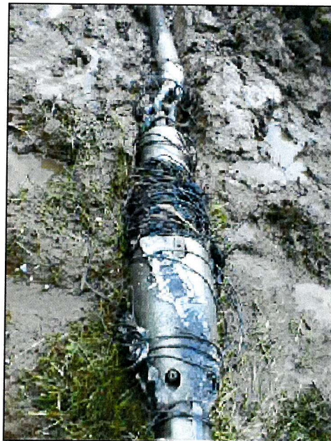
Figure 4.56 Smooth reamer wrapped in wire after well screen installation.
