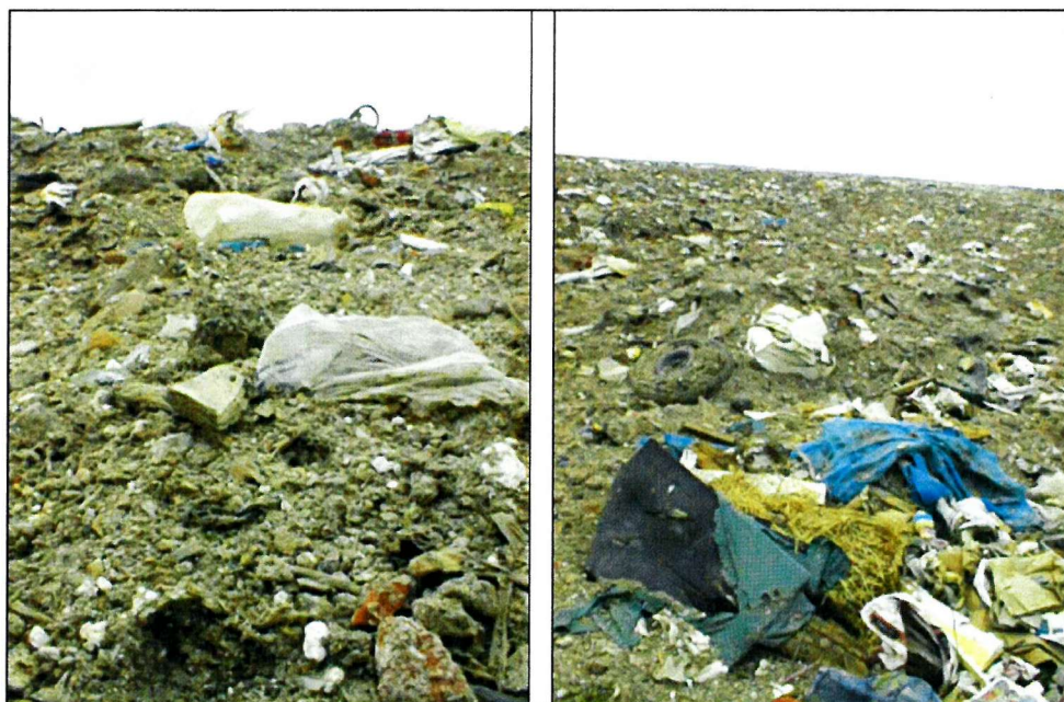
Figure 3.11 The layer of daily cover is rarely complete and unbroken but will have significant effects on the permeability of the waste [Rainham, 2000].
