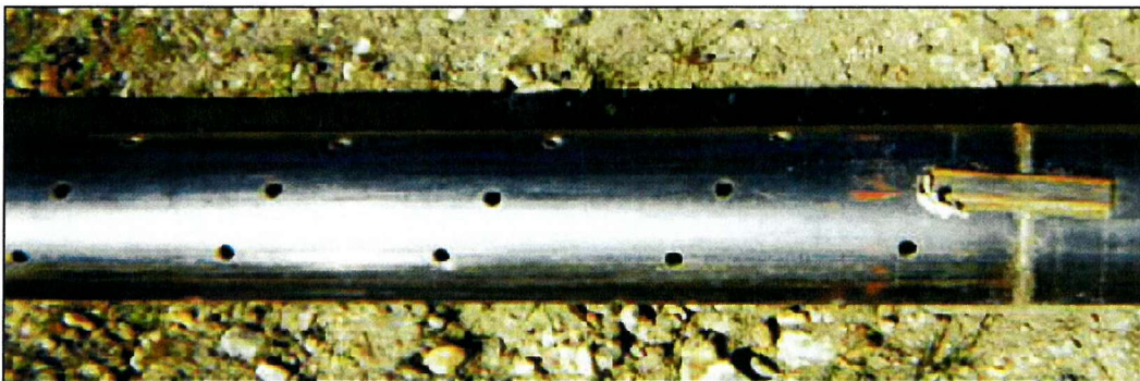
Figure 4.7 150mm diameter well screen used in the first Rainham trial. 15mm holes, open area of 1.5%.
