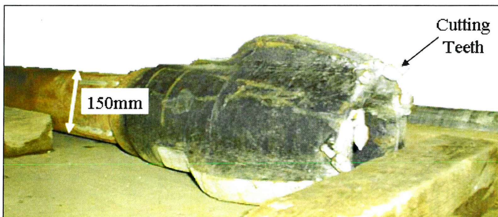
Figure 4.19 Overwash cutting bit, internal diameter 150mm, shows protruding cutting teeth.
