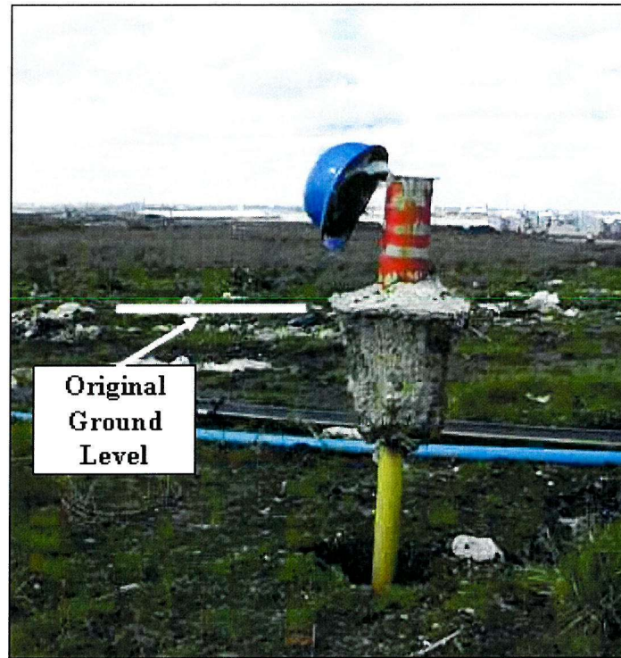
Figure 6.41 Settlement left the piezometer covers well above ground level (HW1C shown).
