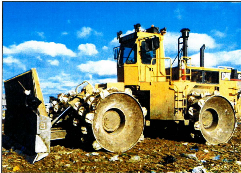
Figure 3.8 Landfill Compactor weighing 54 tons [Rainham, 1998]
