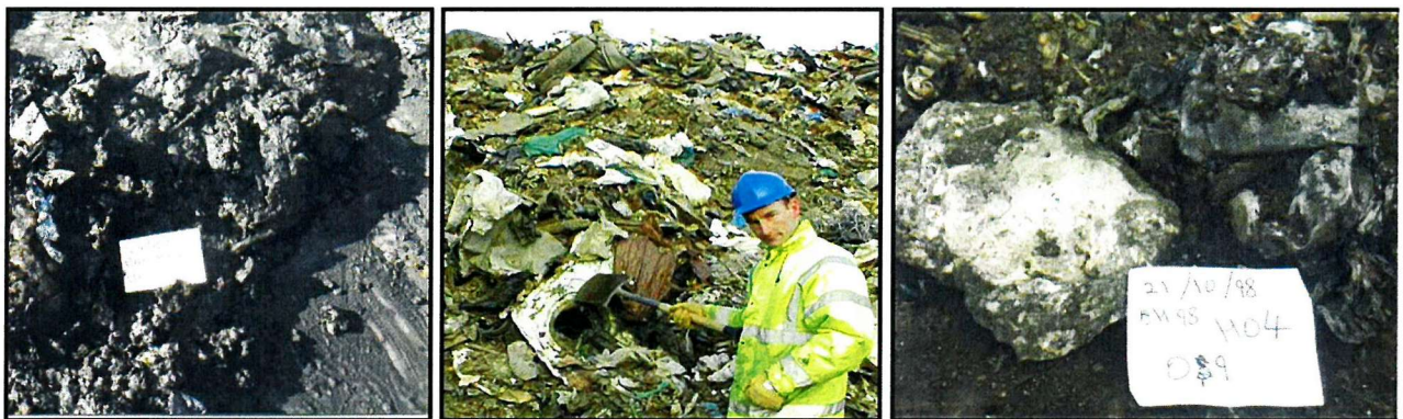
Figure 1.3 Heterogeneity of waste, (a) slurry, (b) discarded washing machine, (c) concrete and steel [Rainham 1998 – 2000]
