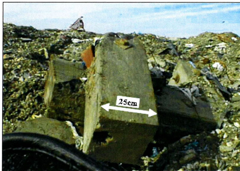
Figure 3.22 Large wooden blocks are present at all depths within the waste [Rainham 1998].
