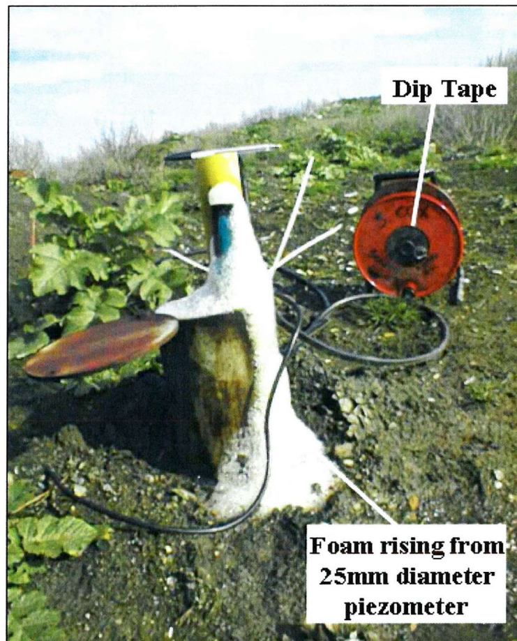
Figure 5.12 Foam rising from piezometer HW3M preventing measurement of the leachate level.
