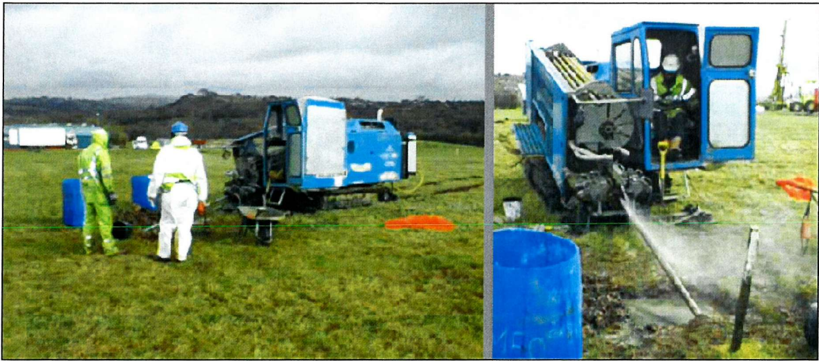
Figure 4.48 Mini-rig at Metallic Tile, 200kN pullback capacity.
