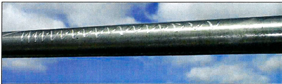
Figure 4.32 Gouges found on the 150mm diameter overwash pipe, caused by hard waste materials.
