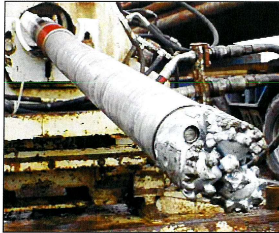
Figure 2.7 Tri-cone drill bit. The angle of the bent sub can be seen [DrillTec, Rainham 2000].
