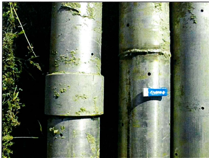
Figure 4.8 100mm diameter steel well screen for the 2 nd Livingston project, 9.5mm holes, open area 0.5%.
