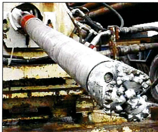
Figure 4.18 Tri-cone reamer that replaced the 'blunt-end' drill bit.
