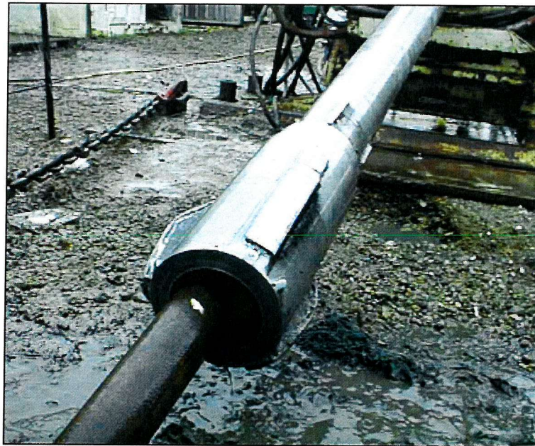
Figure 4.23 Overwash bit had been smoothed from friction with hard waste materials (compare to Figure 4.19)
