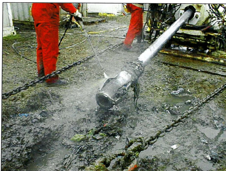
Figure 4.22 Overwash bit wrapped in fabrics and plastics, all cutting teeth had broken off.
