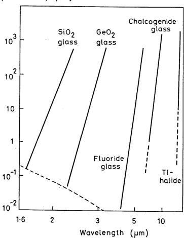
Fig. 7 Calculated loss characteristics of some potential fibre materials. The lower dashed line represents the loss due to Rayleigh scattering.
