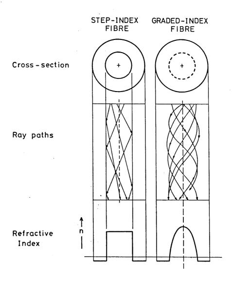
Fig. 5 Ray propagation in step-index, and graded-index, multimode fibres
