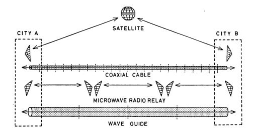
Fig. 3 Microwave Transmission Methods
