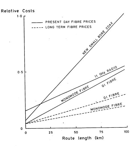
Fig. 6 Cost comparisons of optical fibre systems at 140Mbit/s with digital line and radio systems.
