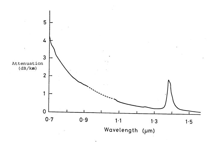
Fig. 4 Spectral attenuation of a high-quality optical fibre
