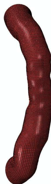
(c) Structured hexahedral element mesh for the first RCA case
