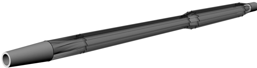
Figure 4.11: A CAD design of a stepped multi-folded balloon model
