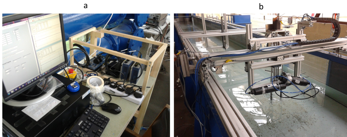
Figure 4.11: Automated ADV positioning rig: (a) PC, drivers and controller, in Chilworth flume working section (b).
