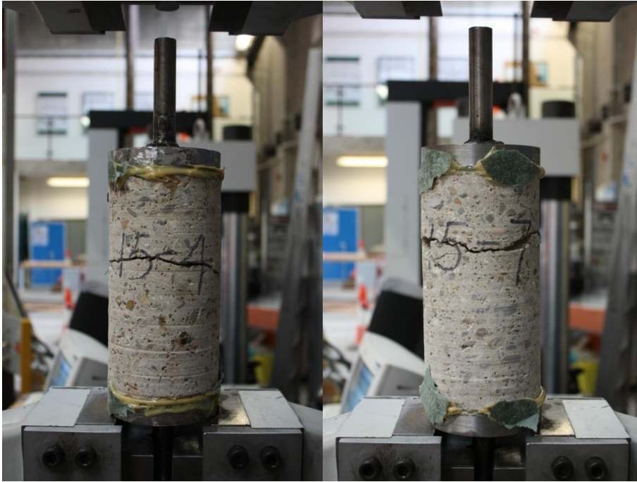
Figure 4-10 Typical failure mode under direct tension tests
