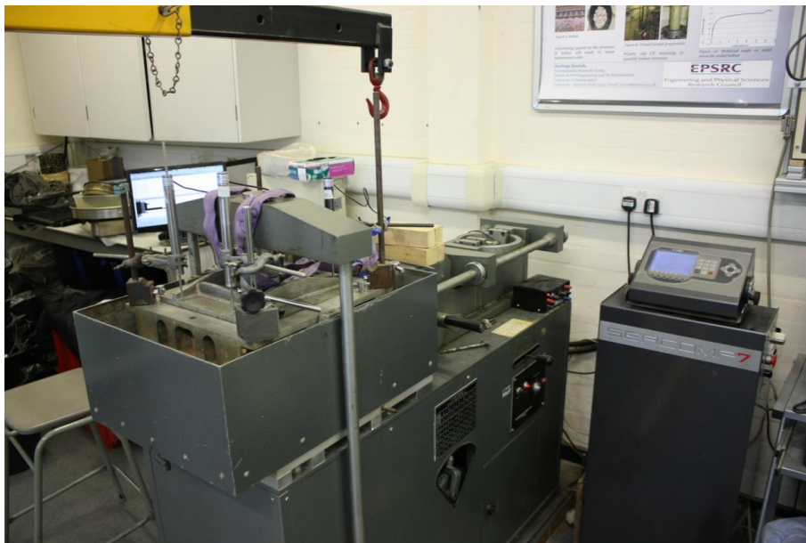
Figure 3–10 Sercomp 7 hydraulic controller system with WF large shear box
