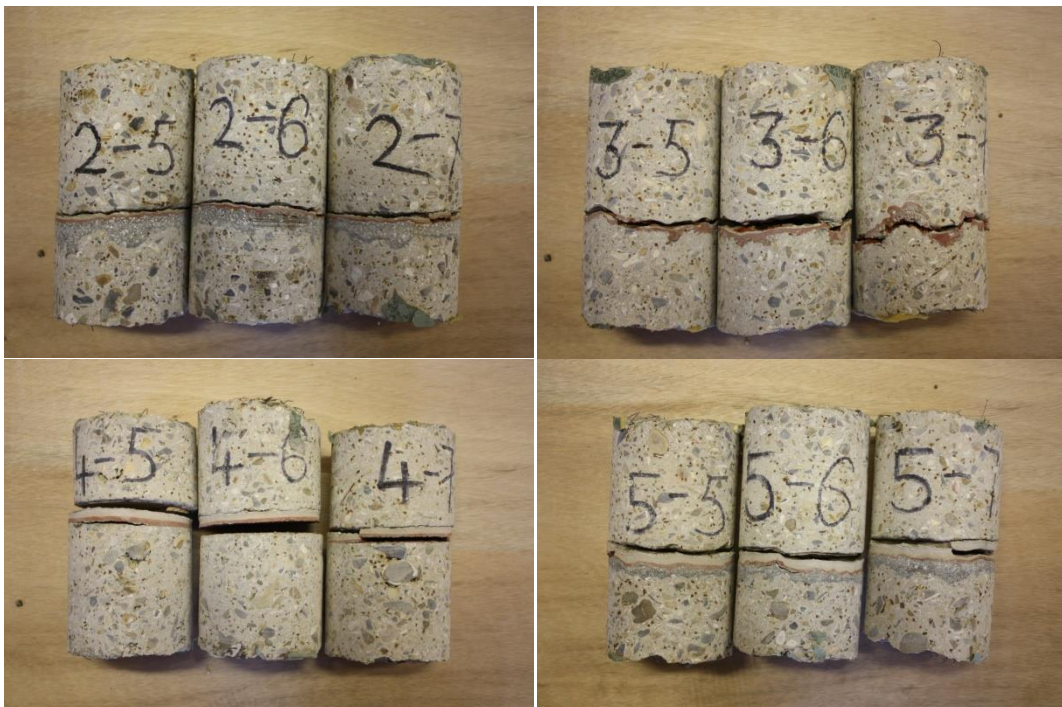
Figure 4–19 Different types of samples with debonded interfaces
