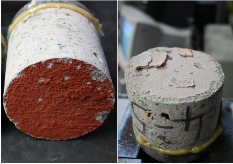
Figure 4–18 Organic/inorganic bond of membrane left on the interface
