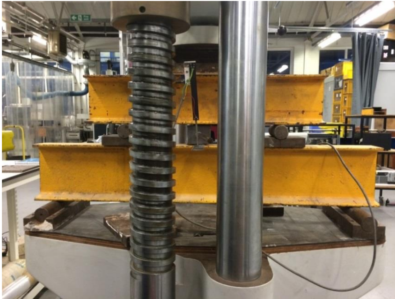
Figure 5–13 Test configuration for the steel beam
