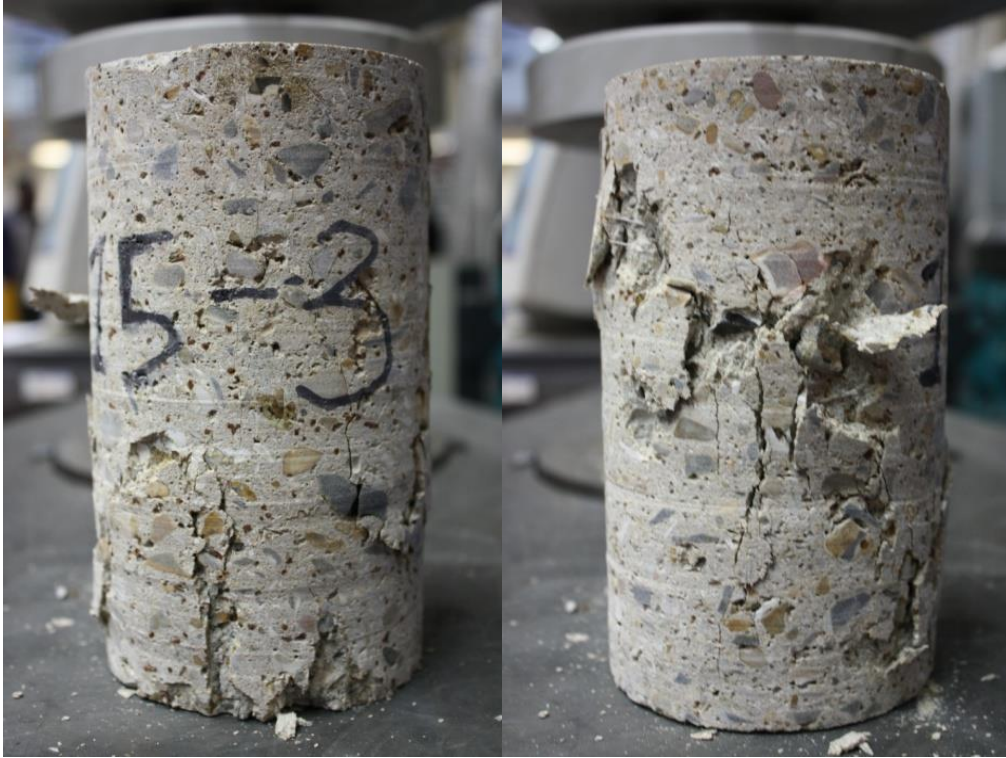
Figure 4-1 Typical failure mode under compression test
