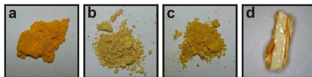
Figure 3. Photographs of selected samples of fluorescein a) flsZ b) flsL :dioxane hemisolvate powder c) flsL :dioxane hemipentasolvate powder, d) single crystal of flsL :dioxane hemipentasolvate. It can be seen that the color of the single crystal is more pale than that of the powder lactoid samples.
