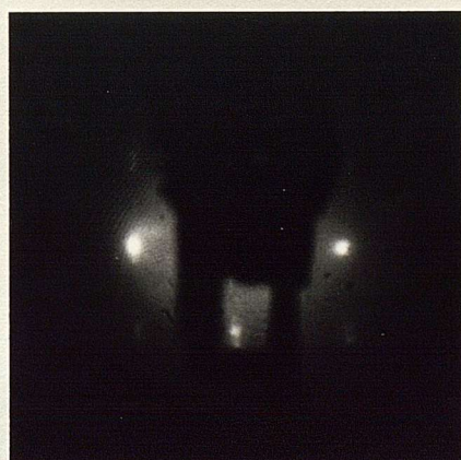
(e) 25V, 15^\circ angle of incidence, (00) left of centre
