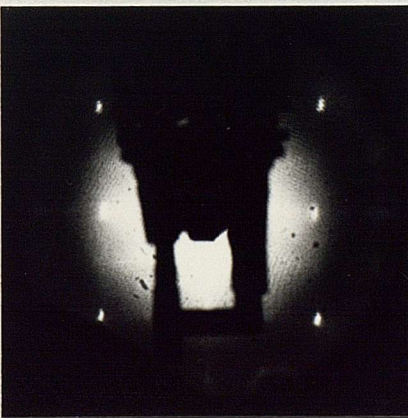
(d) 80.0V Single sharp \{22\} reflections, \{20\} reflections becoming diffuse.
