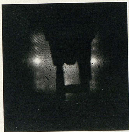
(a) 26.0V Extensive splitting of both the \{10\} reflections and the \{11\} reflections
