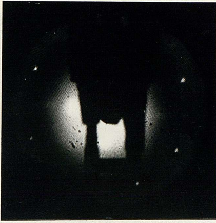
(a) 46.8V Single sharp \{21\} reflections, diffuse \{10\} reflections.
