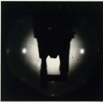
(b) 65.0V No \{21\} reflections visible; \{20\} , and \{22\} reflections diffuse.
