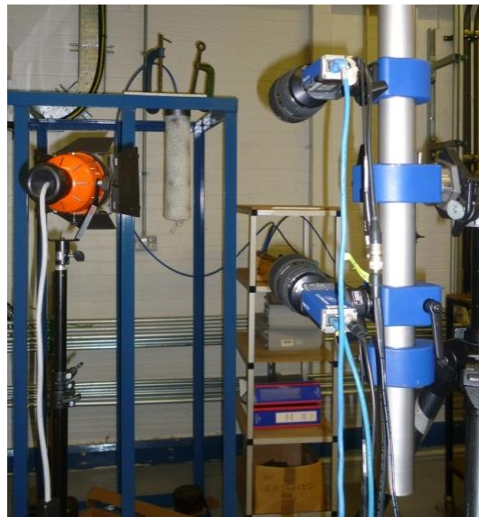
Figure 3.10: The DIC camera and lighting of the inflatable boom biaxial tensile test rig.
