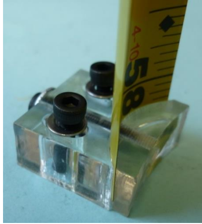
Figure 6.1: Tape spring root clamp assembly.
