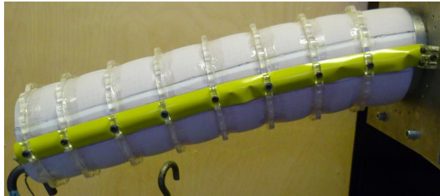
Figure 7.10: Configuration D with 8 evenly spaced attachment collars under 32.8 Nm applied root bending moment at 15 PSI.
