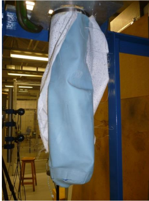
Figure 3.23: Boom failure at 24 PSI with fill yarns orientated in the hoop direction.
