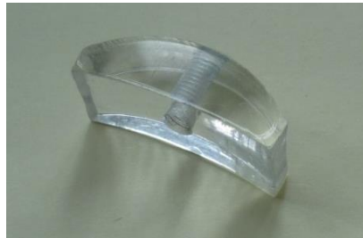
Figure 7.3: Perspex connecting insert with tape spring outer radius and boom inner radius.
