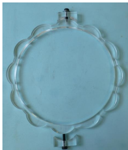
Figure 7.5: Perspex collar and tape collar clamps.
