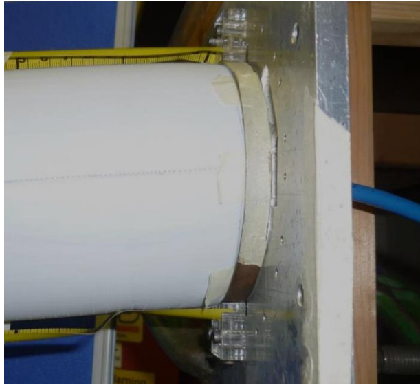
Figure 8.6: 15 PSI configuration B experimental hybrid boom at peak moment.
