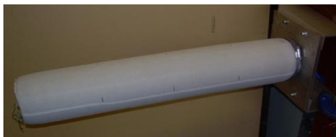
Figure 2.20: Setup of inflatable boom attached at base plate.
