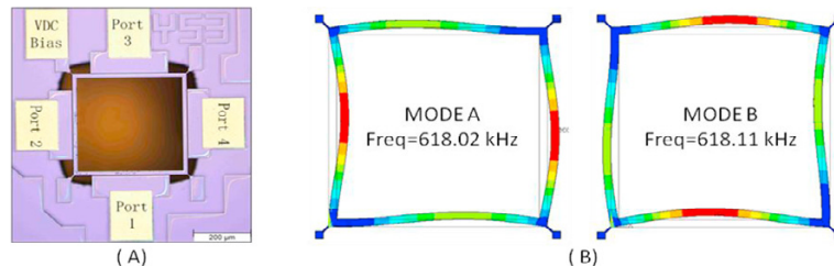
Fig. 1. (A) Optical micrograph (15 μm beam width) and (B) simulated neighbouring mode shapes and natural frequency (ANSYS 11.0)
