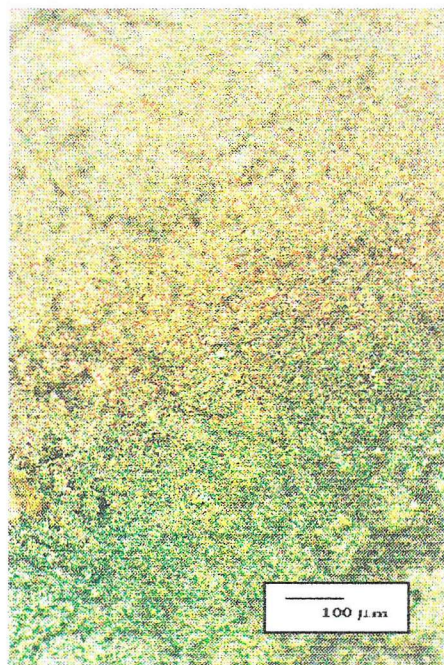
Figure 3.14 - Basal plane of OPC after cycling in PC-based electrolyte
