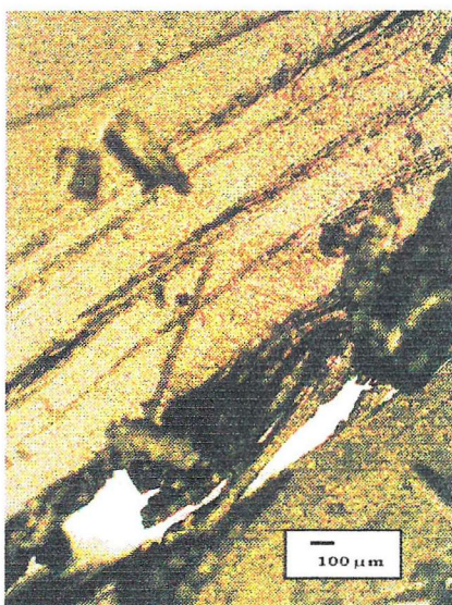
Figure 3.15 - Edge plane of OPC after cycling in PC-based electrolyte
