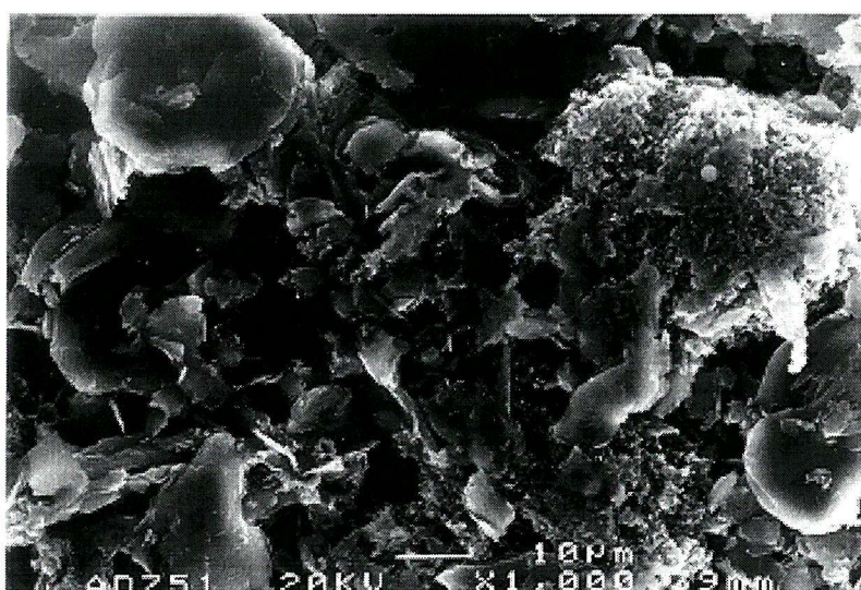
Figure 4.20 - Scanning electron microscopy image of a 5 w/o EPM electrode
