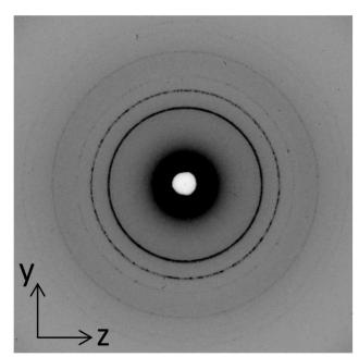
**Figure 5.** SAXS image taken in the zy plane of a thin lipid film on gold foil substrate dip coated from ethanol and 30% phytantriol solution displaying  $Q_{\parallel}^{D}$  phase.
