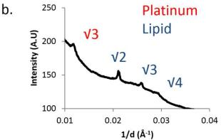
**Figure 6.** (a) SAXS image taken in the zy plane of the platinum nanostructure after deposition and submerged in water before lipid template is removed. (b) Radial profile of the total image with the platinum and lipid peaks Bragg peaks labelled. Limitations in setup resulted in large amount of air scatter which produced a shadow on the top right.
