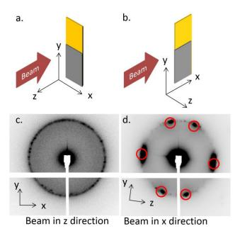
**Figure 2.** Schematic of in-plane and out-of-plane measurements (a – b) with representative images of nanostructured platinum film measured in each configuration (c-d). Predicted scattering pattern for a structure with a Fd3m morphology with the (111) plane orientated parallel to the substrate has been superimposed as circles on image (d).
