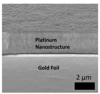
**Figure 3.** SEM image of a platinum nanostructure deposited onto a gold foil substrate. Image was captured in the zy plane with EDX used to confirm platinum and gold regions.
