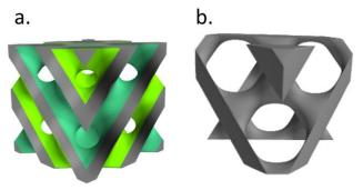
**Figure 1.** (a)  $Q_{ll}^{\ \ D}$  'double diamond' phase where grey region is occupied by lipid bilayer, (b) corresponding 'Single diamond' platinum structure.
