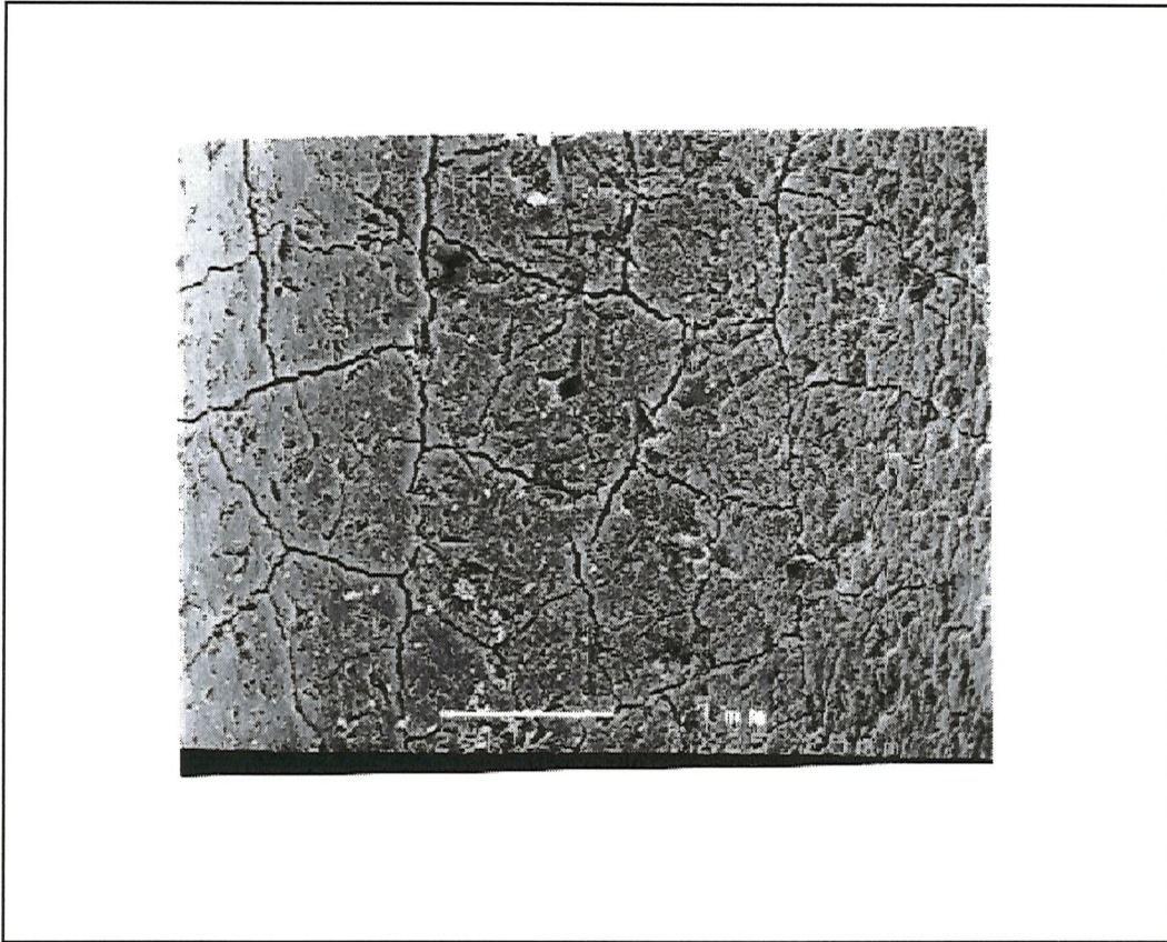
Fig. 3.16 Frit with visible structures after immersion in doping solution (scaling bar : 1 mm)
