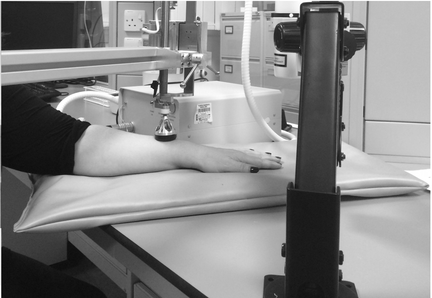
Fig. 2. Example mechanical loading over the volar aspect of a participant's wrist.
