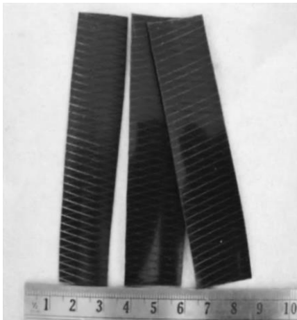
Figure 2. Polyethylene fibres (or strips) used in the triaxial tests
