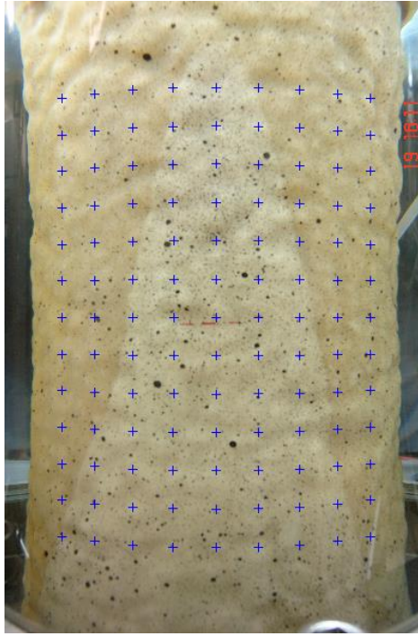
Figure 5. Typical image of a triaxial specimen captured during shear, showing grids used for image-based deformation measurement and the speckled pattern on the membrane
