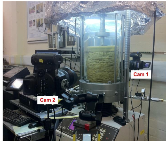
Figure 4. The triaxial setup for image-based deformation studies showing a triaxial specimen in the transparent cell during shear, cameras positioned at angular distance of \sim 120^\circ , uniform light source and light reflecting curtain (which is in a raised position in this image)
