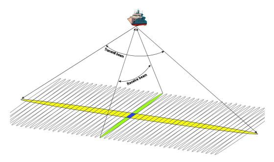
Figure 1.5: Visualisation of a multibeam echosounder sending out an array of sound pulses in a fan shape, then the beams bounce off the seabed and returns depths from underneath to the ship where the echoes are recorded. (Source: AML Oceanographic)
