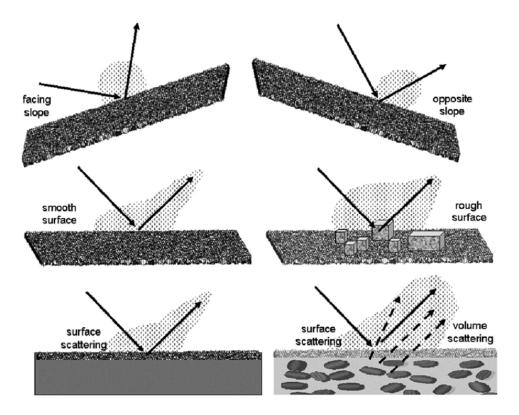
Figure 1.8: Backscattering is affected by three factors with decreasing order of importance: 1) geometry of the sensor-target system (local angle of incidence of the sonar beam, local slope), 2) physical characteristic of the surface (roughness of the seafloor at scales comparable with sonar's wavelength) and 3) intrinsic nature of the surface (e.g., rocks vs. sediments) (Source: Blondel, 2009)
