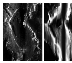
Figure 1.11: On the left is a section of real sidescan sonar imagery acquired through sonar survey in a submarine canyon. Meanwhile, image on the right is a synthetic sonar imagery produced by simulating the flight of the sonar onto multibeam bathymetry data of the same area. Synthetic imagery contains topographical and slope attributes without any lithological effect in comparison to real sidescan sonar imagery. Topographical features can be clearly seen and matching between the two images.
