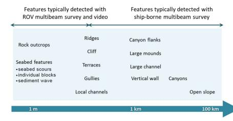
Figure 1.3: Some of the typical seafloor features that can be mapped by ship borne and ROV multibeam bathymetry.
