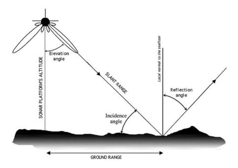
Figure 1.7: Components of an echo event on the seafloor (Source: Blondel, 2009)
