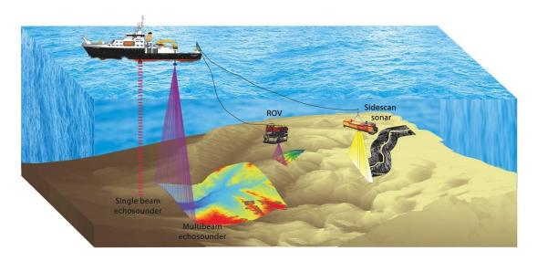
Figure 1.4: Illustration of the common acoustic systems used during seabed surveys. ROVs can be equipped with video, camera and a multibeam system. This thesis uses acoustic data acquired from ship-borne and ROV-mounted multibeam bathymetry and sidescan sonar system.
