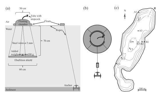
**Figure 1.** (a) Schematic representation of our adaptations to the floating chamber design presented by *Cole et al.* [2010]. (b) Top view of our shielded floating chamber setup. (c) Bathymetric map of Lake Gerzensee showing the locations of the sampling stations. The numbers indicate the depths of the isobaths, and the cross marks the location of the weather station.
