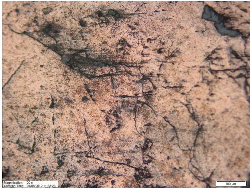
**Figure 4.60:** Optical microscopy picture of  $\text{MgB}_2+2 \text{ wt}\% \text{ C}+16 \text{ wt}\% \text{ SiO}_2$ .
