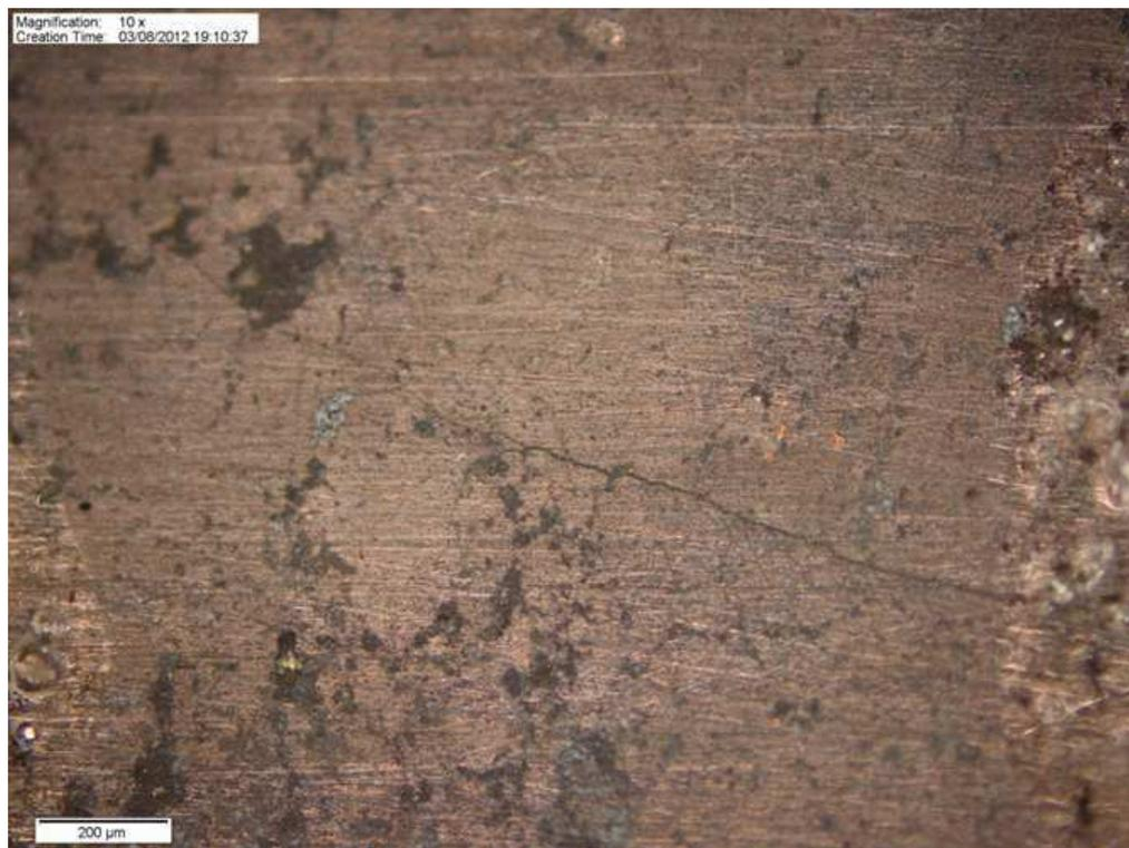
**Figure 4.14:** Optical microscopy image of C-CVD doped MgB<sub>2</sub> treated at 850°C.
