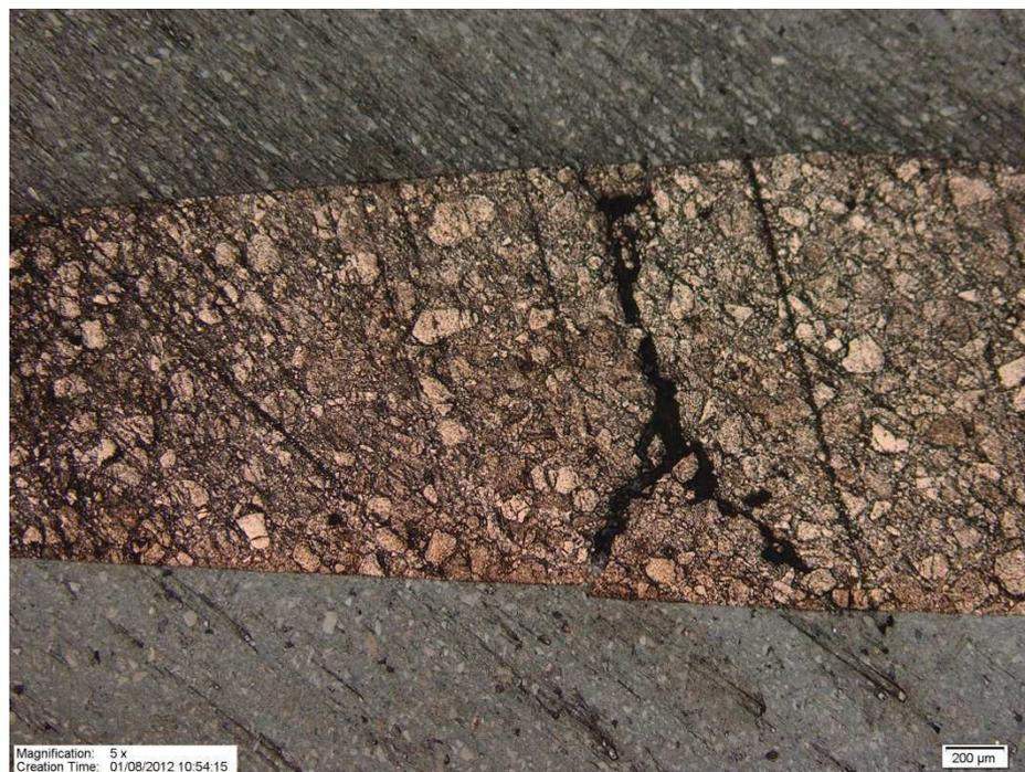
**Figure 4.10:** Optical microscopy image of the undoped  $\text{MgB}_2$  treated at  $850^\circ\text{C}$ .
