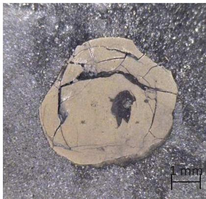
**Figure 4.7:** MgB<sub>2</sub> bulk sample sintered at 900°C for 6 hours, using a heating rate of 10°C/h.
