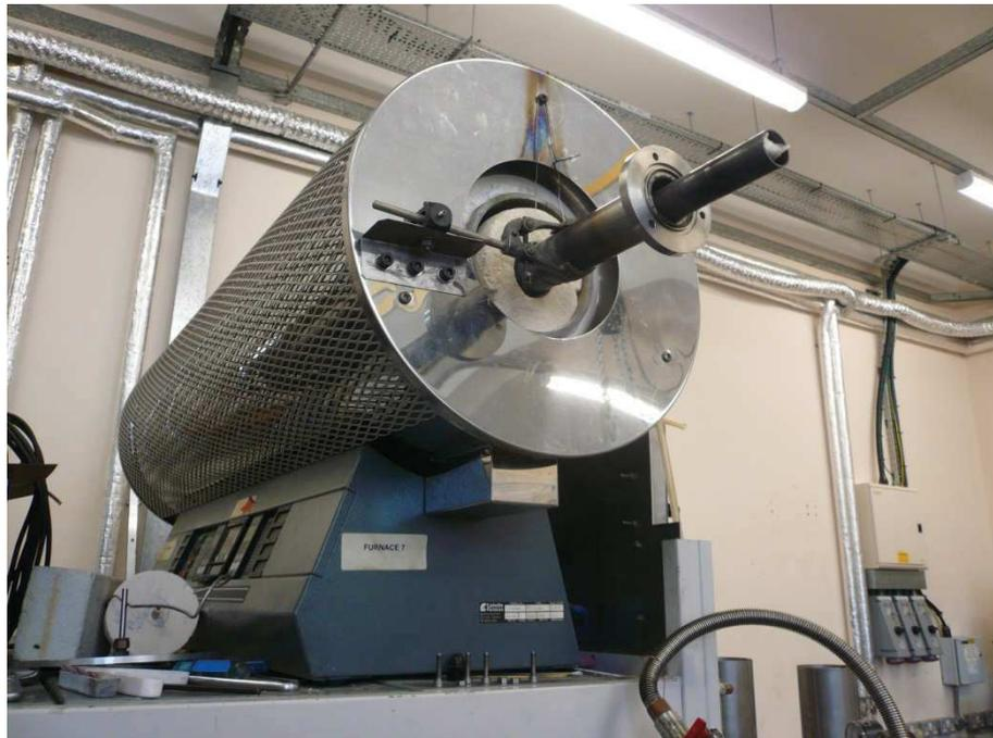
**Figure 3.2:** Tube furnace used to react  $\text{MgB}_2$  powder samples.
