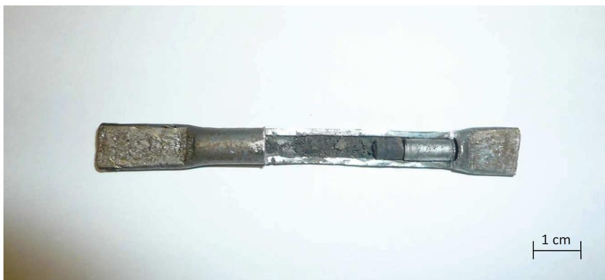
**Figure 4.16:** Optical microscopy picture of MgB<sub>2</sub> bulk sample showing the presence of well-reacted and dense areas, which are located in the proximity of the original position of the magnesium rod, and powdery sections of the sample, which are poorly reacted and sintered.
