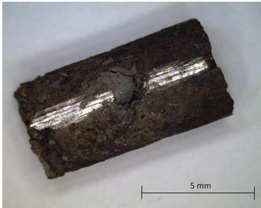
**Figure 4.9:** MgB<sub>2</sub> bulk sample sintered at 970°C for 6 hours starting with a mixture of Mg, B and MgB<sub>2</sub> (molar ratio of (Mg+2B):MgB<sub>2</sub>=1:1).
