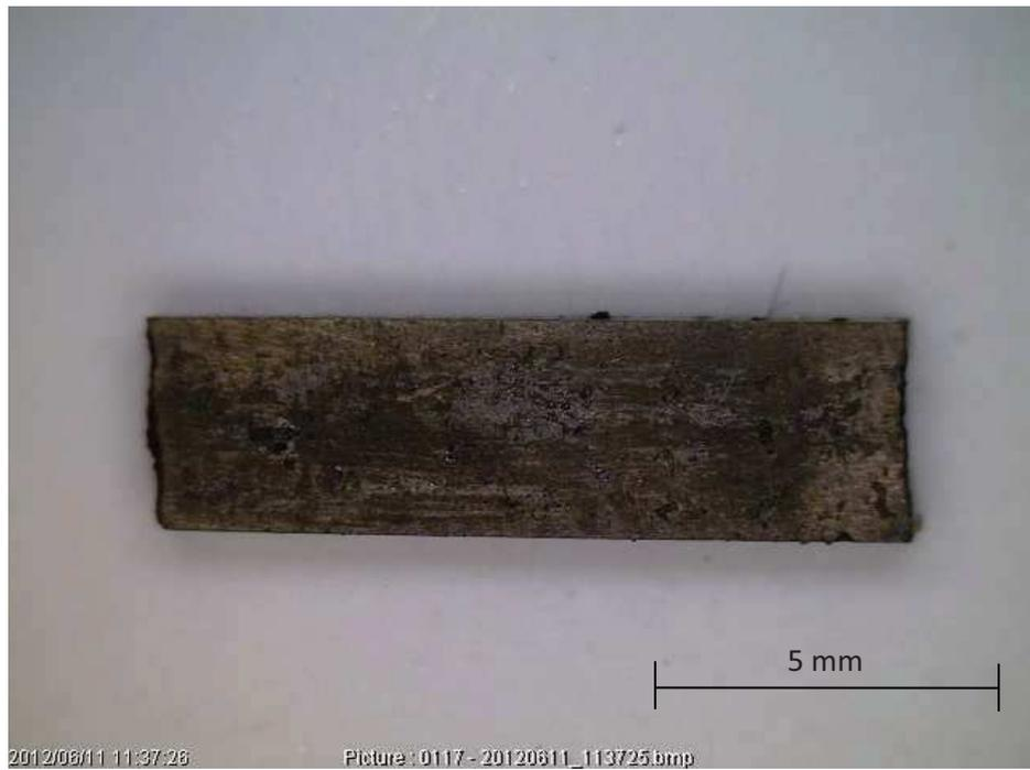
**Figure 4.11:** Optical microscopy image of the undoped MgB<sub>2</sub> treated at 775°C.
