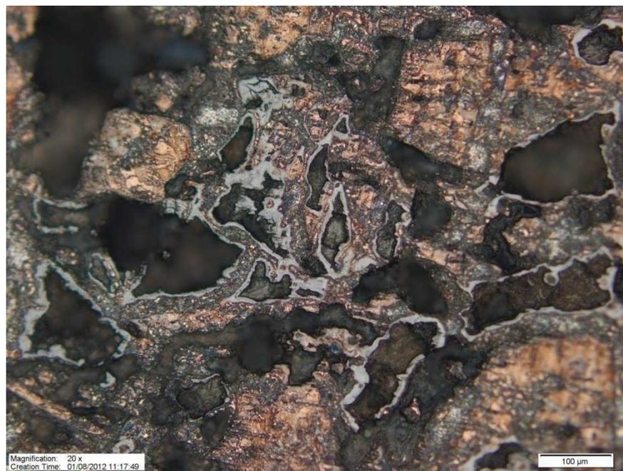
**Figure 4.59:** Optical microscopy picture of MgB<sub>2</sub>(C - 6.1 wt%)+16 wt% SiO<sub>2</sub>.
