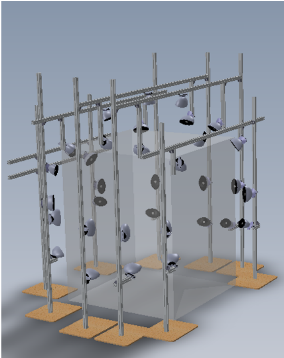
Figure 4.2: The supporting structure simulated in Solidwork. The gray cube represents the isolation booth used for the subjects.
