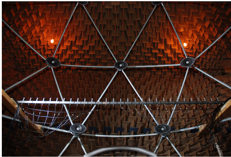
FIGURE C.2: Measurement of the acoustic field produced by a 5th order Ambisonics system
