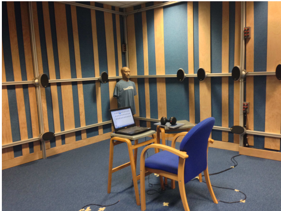
FIGURE 3.38: Audio-Lab, set up of the listening test
