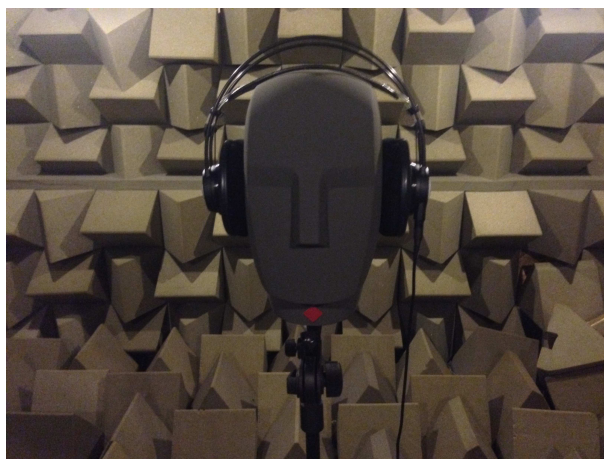
FIGURE 6.2: Measurement of headphone frequency responses, AKG K-702
