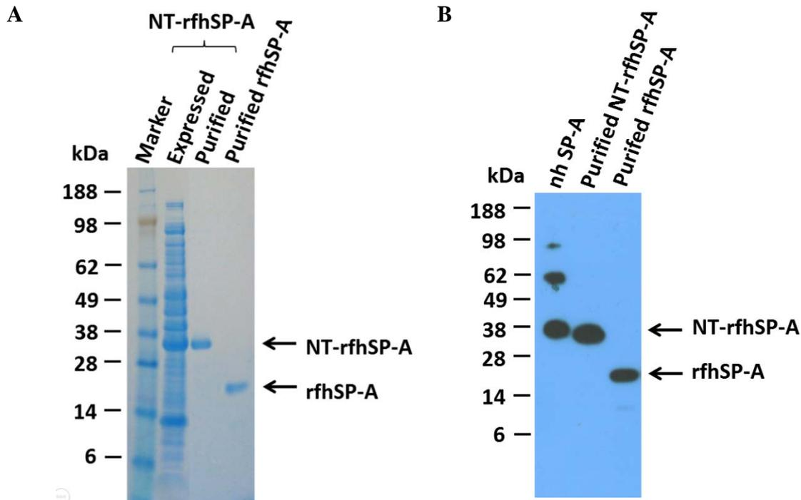
**Figure 5-6: Removal of NT and purification of rfhSP-A.** Samples of expressed and purified NT-rfhSP-A and purified rfhSP-A after cleavage were analysed by SDS-PAGE with subsequent Coomassie staining (A) or Western blotting using an antibody against nhSP-A (B). Purification was undertaken with the increased stringency using 20mM imidazole and 500 mM NaCl upon loading protein and washing the nickel affinity column. Indicated are bands corresponding to NT-rfhSP-A and rfhSP-A.
