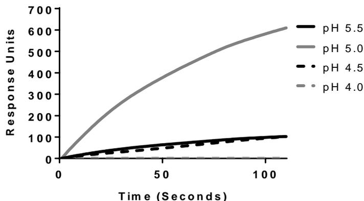
**Figure 7-4: Optimisation of conditions for optimal immobilisation of rfhSP-A to a Biacore chip.** The capacity of rfhSP-A to bind to a Biacore sensor chip was tested in 10 mM sodium acetate buffer over 120 seconds at different pH values: pH 5.5, 5.0, 4.5 and 4.0. The level of immobilisation is shown as measured by level of response units.
