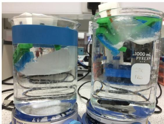
**Figure 6-3: Impact of redox glutathione on precipitation.** Shown is an image of the protein precipitation after completion of refolding and dialysis into TBS without urea. The precipitation was compared between the normal refold protocol (left) and that using the oxidized and reduced glutathione refold system (right).
