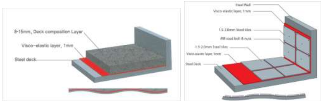
Figure 1.3 Examples of PCLD treatment application in industry [www.dae-hyup.com/en_product_02_18.html]
