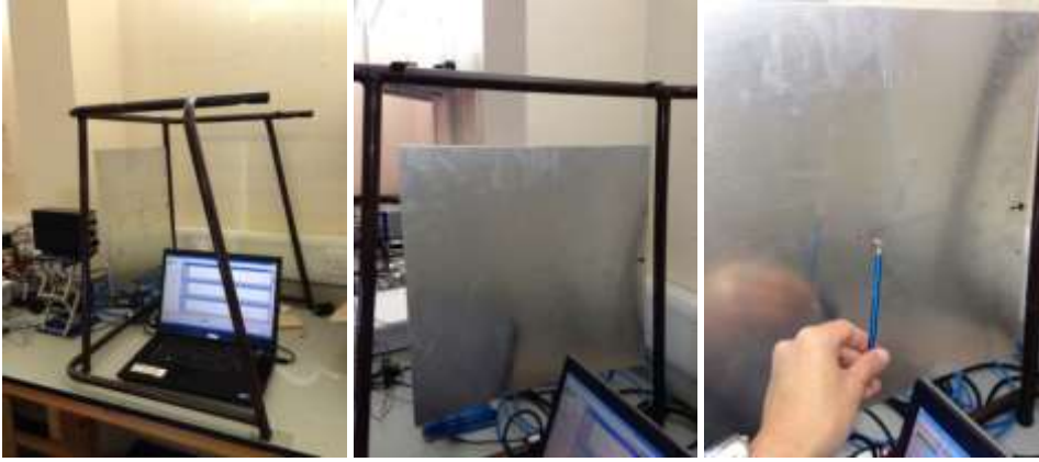
Figure 7.7 Impact hammer test for a singly curved plate
