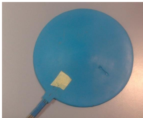
Figure 3.4 SIT-pad with an integrated tri-axial accelerometer (Willow Technologies KXD94-2802).
