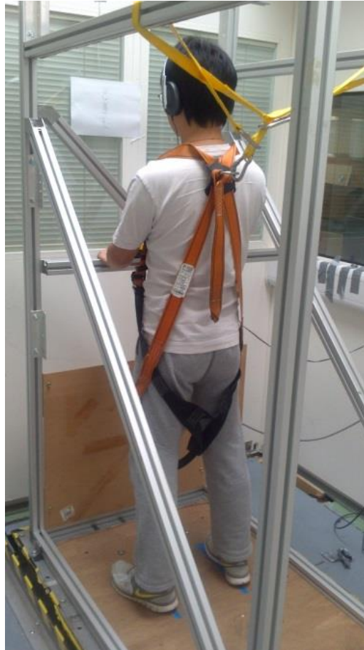
Figure 3.8 Equipment used to secure and protect the subject during the experiment investigating discomfort whilst standing.
