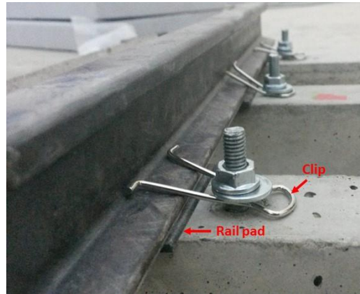
Figure 7.1 Fastening system in the measurements
