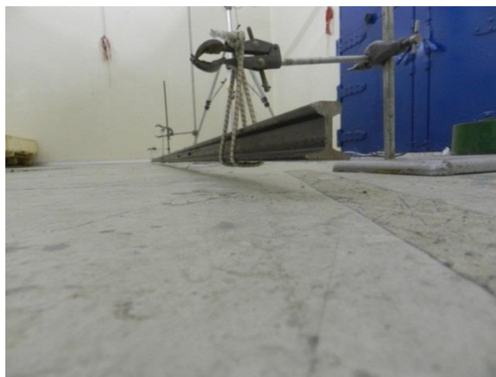
Figure 6.11 Rail suspended above rigid ground
