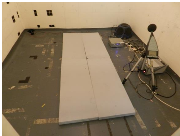
Figure 5.11 Experimental set-up for four pieces of melamine foam
