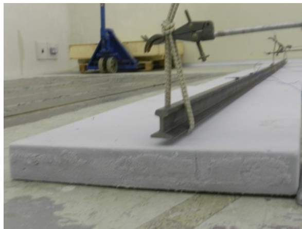
Figure 6.13 Rail 20 mm above absorptive material
