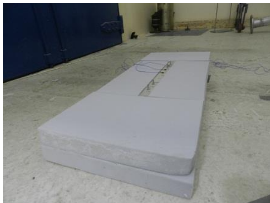
Figure 6.22 Sleeper embedded in melamine foam
