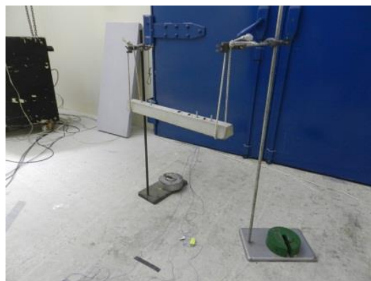
Figure 6.16 Freely suspended sleeper
