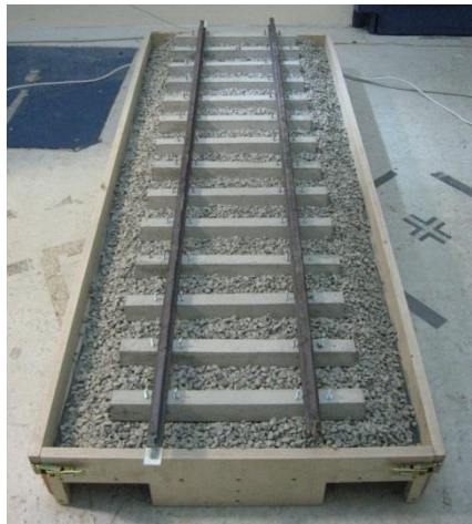
Figure 6.1 1:5 scale model track [89]
