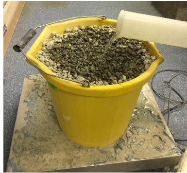
Figure 5.7 Measurement of the porosity of the scale ballast
