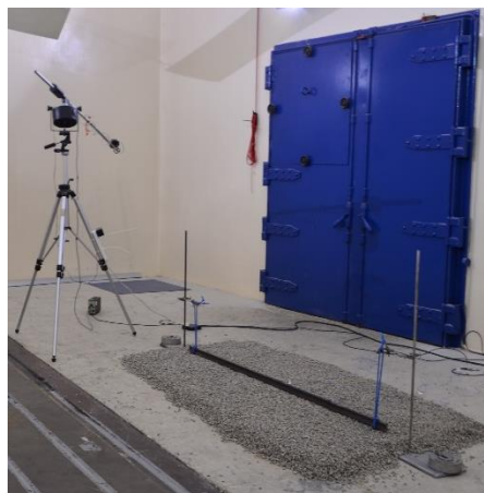
Figure 6.30 Rail 20 mm above the scale ballast on the rigid ground
