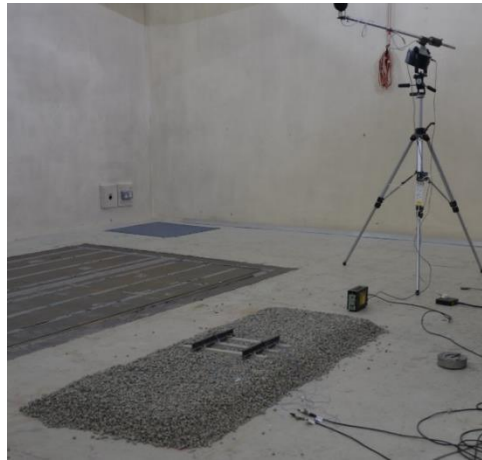
Figure 6.35 Experimental set-up for three sleepers embedded in ballast
