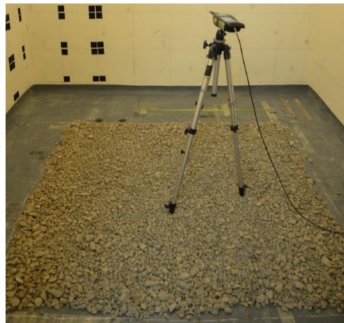
Figure 5.14 Experimental set-up for the 1:\sqrt{5} scale ballast
