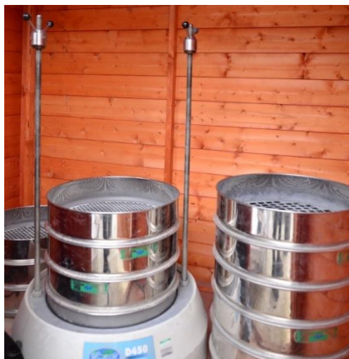
Figure E.1 Sieving machine (D450 Endecott Shaker) with different sieve sizes
