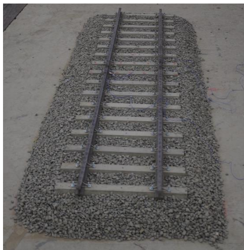
Figure 7.8 Experimental set up for the scale whole track embedded in ballast
