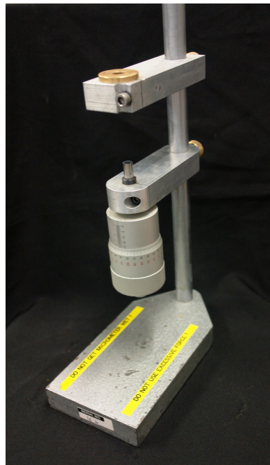
Figure B.1: Mitutoyo series 152-348 micrometer used for displacement calibration of LVDTs, 25 mm range and 1 \mu\text{m} resolution
