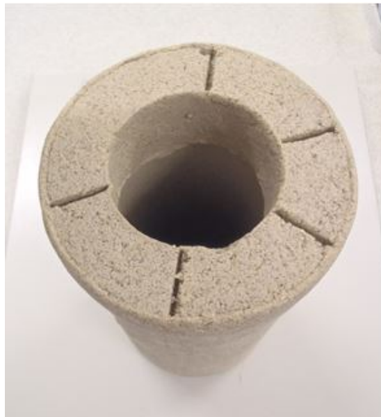
Figure 4.25: Cuts made into the top surface (similar for the bottom) of the HCA specimen at the positions of the porous disc fins
