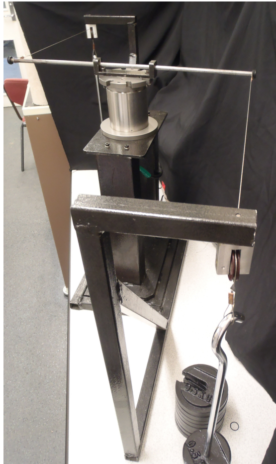
Figure B.3: Dead-weight calibration frame built by Gräbe (2002) used for the torque calibration of the HCA combined load&torque transducer
