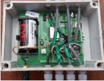
Figure 1. Wireless strain sensor node developed in CSIC
