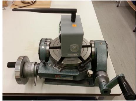
(a) Tilt sensor calibration platform
