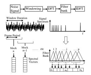
Fig. 1 – Frequency Selective mechanism for noise identification
