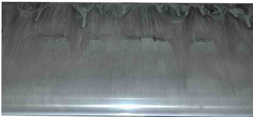
Figure 6.23: surface flow visualisation h/c=0.25 . Mid-span suction surface viewed with leading edge at the bottom of the image.
