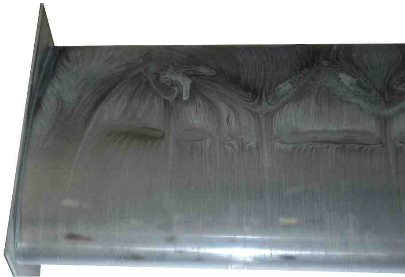
Figure 6.28: surface flow visualisation h/c=0.08 . Suction surface viewed with leading edge at the bottom of the image.
