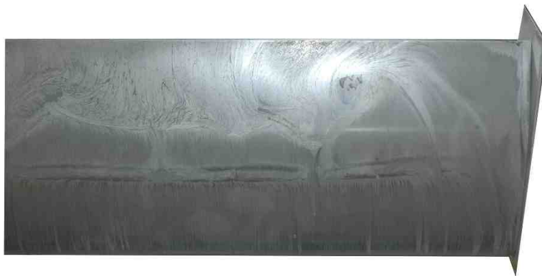
Figure 6.27: surface flow visualisation h/c=0.08 . Righthand suction surface viewed with leading edge at the bottom of the image.
