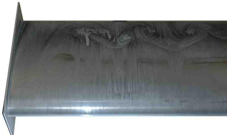
Figure 6.25: surface flow visualisation h/c=0.1 . Suction surface viewed with leading edge at the bottom of the image.
