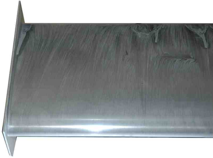
Figure 6.22: Surface flow visualisation h/c=0.25 . Suction surface viewed with leading edge at the bottom of the image.
