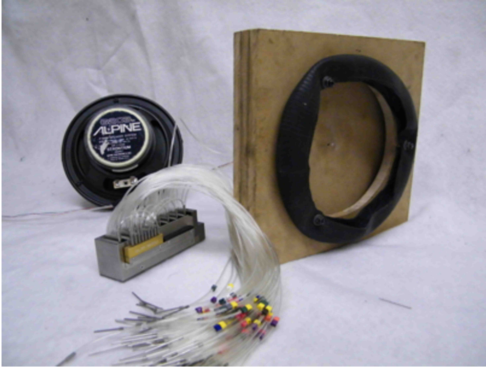
Figure 4.7: Pressure sensor, calibration chamber, speaker and Zoc33 module.
