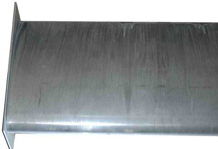
Figure 6.21: Surface flow visualisation at h/c=1 . Suction surface viewed with leading edge at the bottom of the image.
