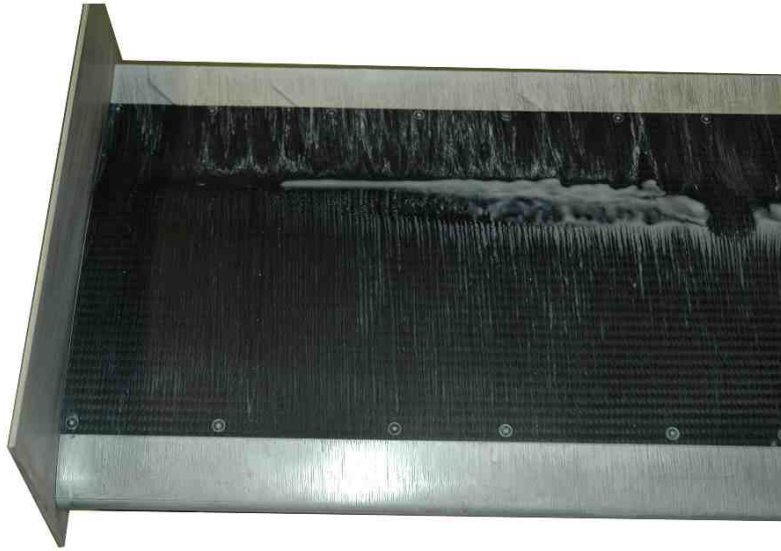
Figure 6.20: Surface flow visualisation at h/c=1 . Pressure surface viewed with leading edge at the bottom of the image.
