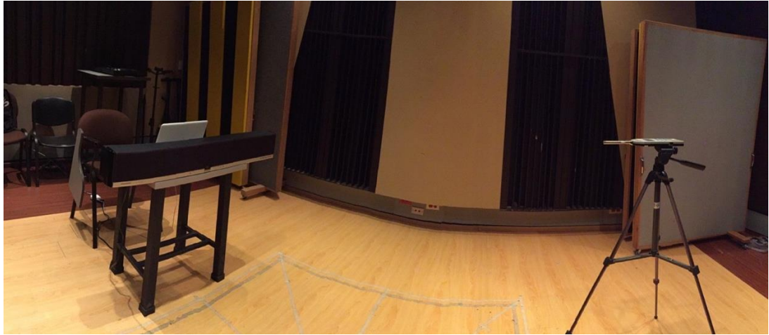
Figure 6.8: Measurement set up to include noise in the auralizations.
