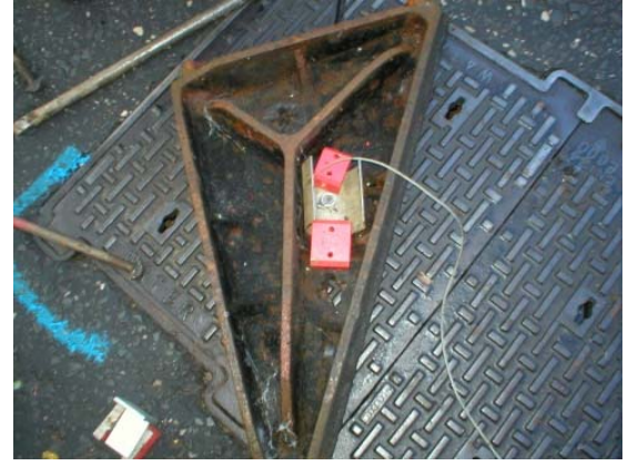
Fig. 2. An accelerometer attached to a manhole cover.
