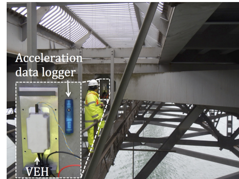
Figure 6: Photograph of the deployment trial testing using the VEH prototype powering a WSN mote. This particular location illustrates testing on the cross girder underneath the deck of the Forth Road Bridge.
