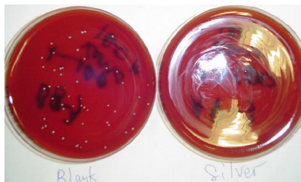
Figure 8: Photograph of two agar plates in contact with Staphylococcus aureus solutions. The reference sample on the left shows growth of bacterial colonies while the right, which also contains a silver-silicon carbonitride composite, is free from colonies. Reproduced with kind permission from [92].
