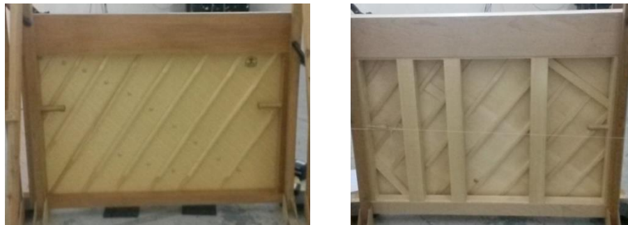
Figure 2. Laminated soundboard (left) and Tone-wood soundboard (right).
