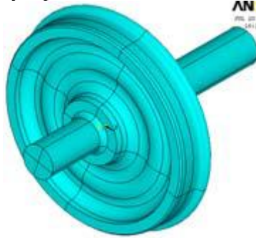
Figure 6. Solid model of Class 158 wheel
