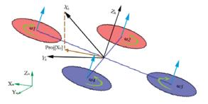
Fig. 2 Coordinate system and quadrotor setup
