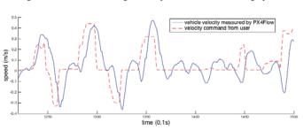
(a) Short-term command-response graph of velocity in x-axis in match-heading frame
