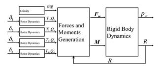
Fig. 3 Overview of the quadrotor dynamics model
