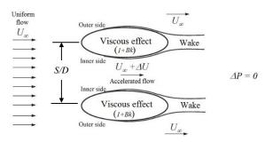
Figure 1: Flow past twin hulls in parallel configuration
