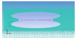
Figure 5: Fine mesh set on ZX plane at Y = 0 from the centreline with the fluid flow from left to right
