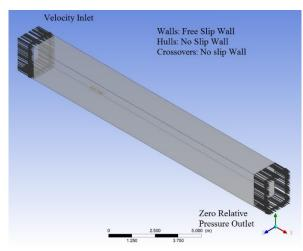
Figure 4: Fluid domain and boundary condition
