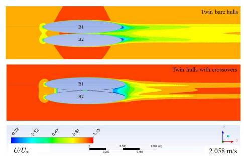
Figure 7: The velocity profile of 2.058 m/s flow past twin hulls with and without crossovers
