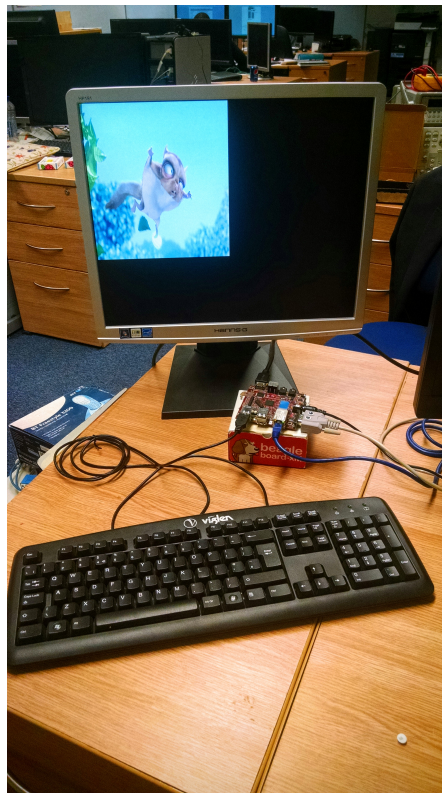
FIGURE 5.2: Video Decoding experiment using Shepherd Governor running on BeagleBoard-xM
