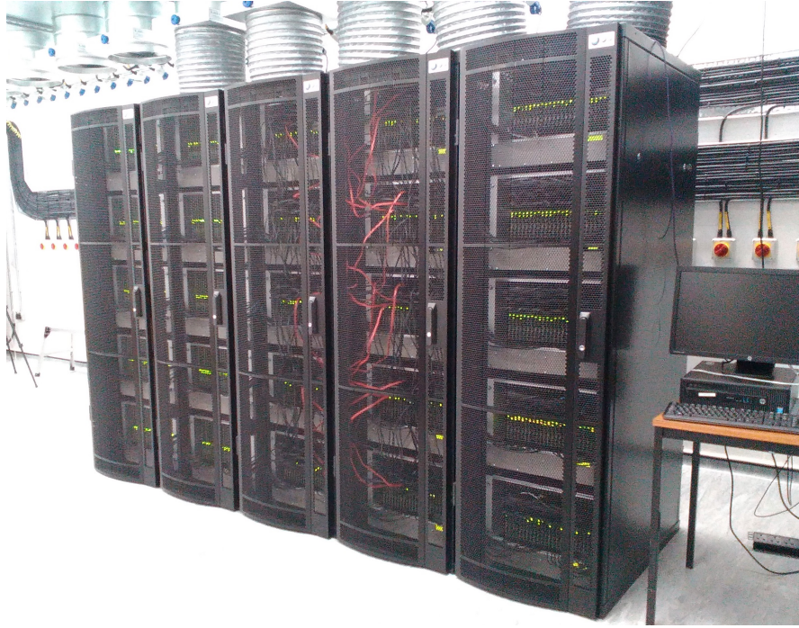
Figure 3.18: Five SpiNNaker-105 cabinets forming the largest SpiNNaker system assembled to date. Each SpiNNaker-105 is built from five SpiNNaker-104 systems for a total of 5,760 chips and 103,680 processors. The system in this picture therefore contains 28,800 chips and 518,400 processors.
