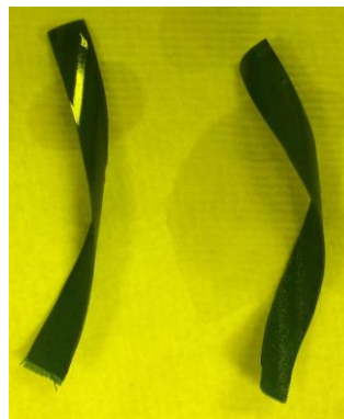
Figure 7.3: Samples of UV-IF-1 coated fabrics after submerging it de-ionized water for 5 minutes
