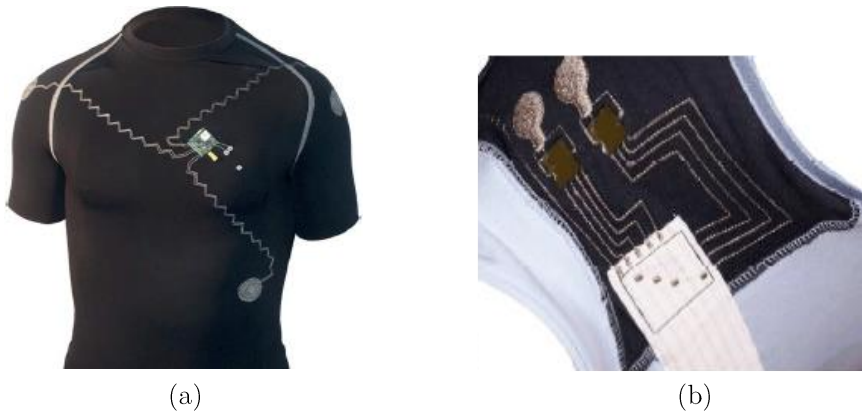
Figure 2.8: (a) Fully integrated EKG shirt with embroidered interconnections [42], (b) Two contactless embroidered sensors integrated into a vest. Wiring was done with embroidery and conductive woven yarns (White ribbons) [44]
