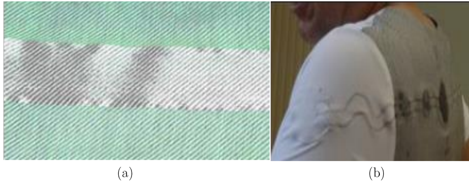
Figure 2.9: (a) Woven stainless-steel wires on fabric used as bus for the VTAMN health monitoring system [45] (b) The embroidered sinusoidal wiring [45]
