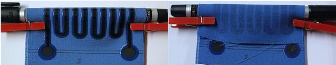
Figure 4.16: Negative bending (left) and positive bending (right) orientations of the strain gauges
