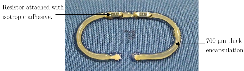
Figure 6.11: Screen Printed resistive circuit on neutral axis on a Bari- textile patch
