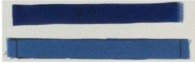
Figure 7.2: Samples of UV-IF-1 coated (top) and uncoated (bottom) fabric samples before testing
