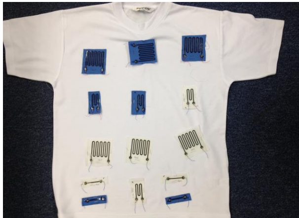
Figure 6.5: Strain gauge patches stapled on a T-Shirt
