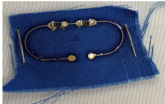
Figure 3.18: The resistors in circuit 3 still firmly attached after 2 nd wash but with discontinuity along the silver conductor
