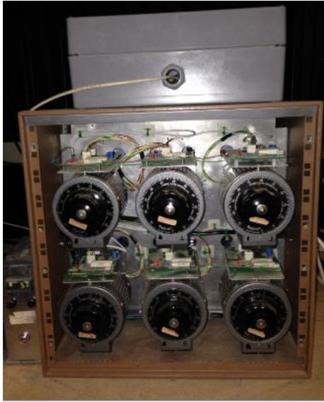
Fig. 113 Front side of variac unit
