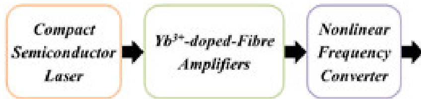
Figure 1-1 Block diagram of the ultrashort-pulse systems to be presented in this thesis
