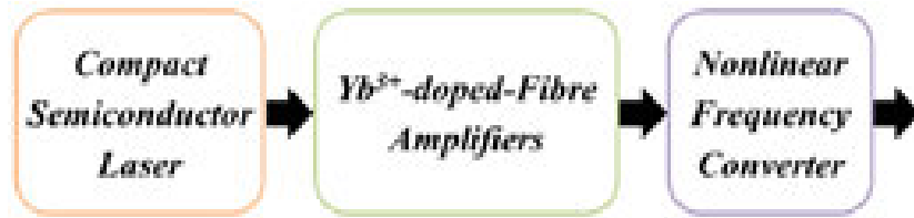
Figure 7-1 Block diagram of the ultrashort-pulse systems presented in this thesis
