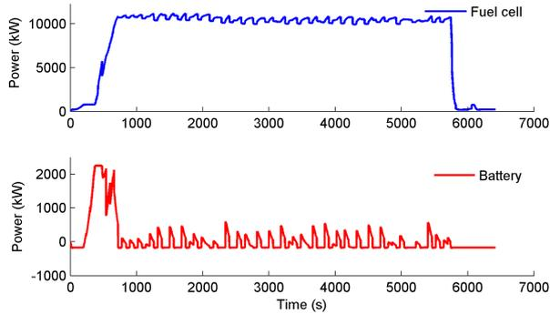
**Figure 14.** Fuel cell and battery power for voyage 1
