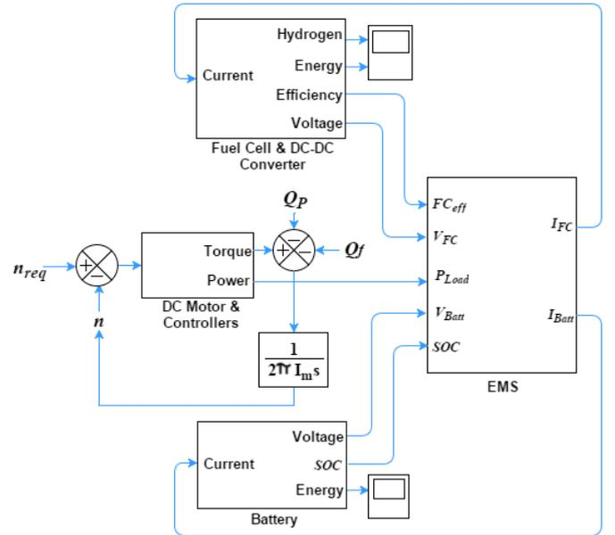
Figure 6. Hybrid fuel cell/battery propulsion system in Simulink/MATLAB environment
