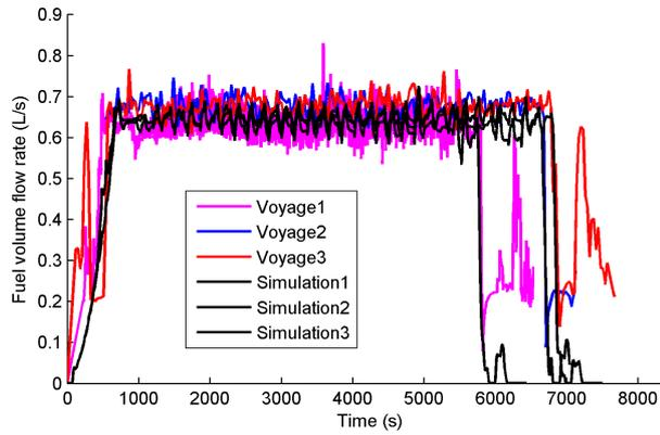
**Figure 11.** Validation of ship fuel volume flow rate simulation result
