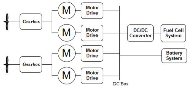
**Figure 3.** Proposed hybrid fuel cell propulsion system
