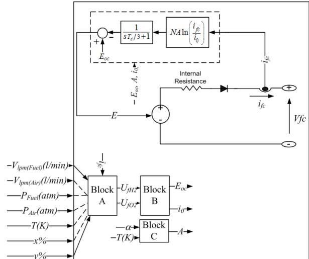
**Figure 8.** Fuel cell model in Simulink/MATLAB environment
