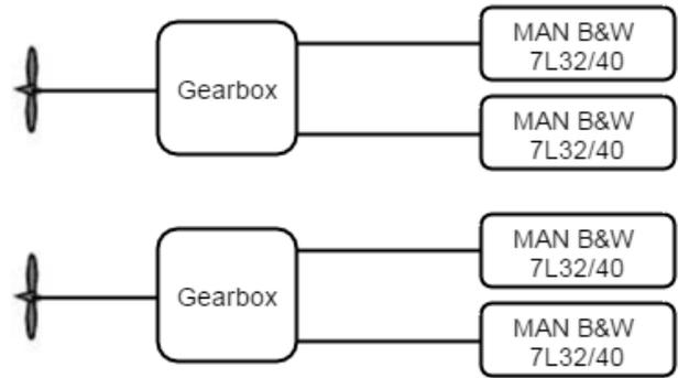
**Figure 2.** Configuration of M/S Smyril diesel propulsion system
