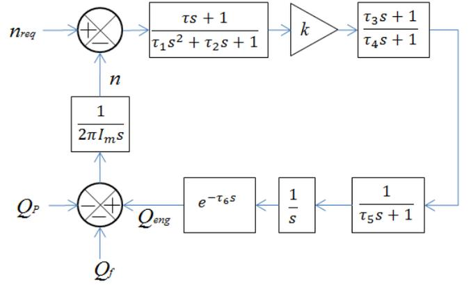
Figure 5. Diesel engine dynamic model
