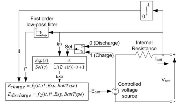
**Figure 9.** Battery model in Simulink/MATLAB environment
