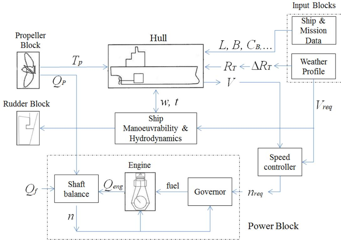
**Figure 4.** Total ship simulator representation using diesel propulsion system
