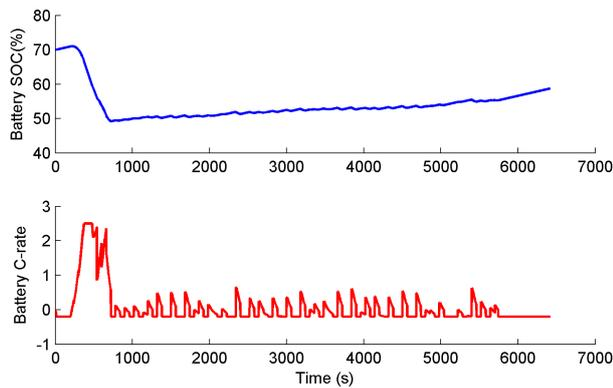
**Figure 15.** Battery SOC and C-rate for voyage 1
