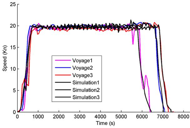
**Figure 10.** Validation of ship speed simulation result
