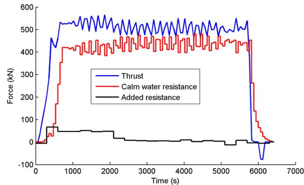
**Figure 12.** Acting forces on the hull during voyage1
