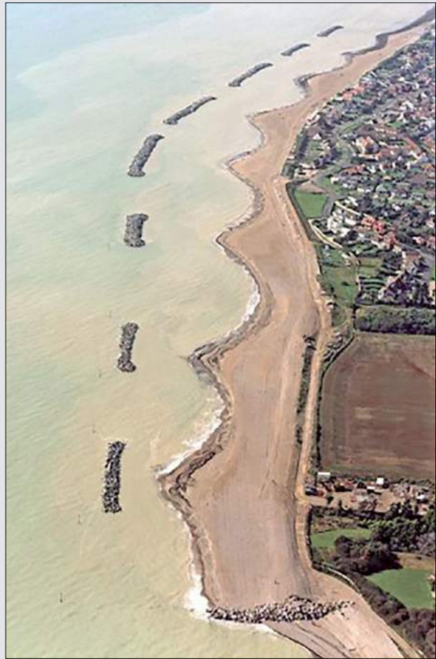
Figure 3 Elmer coastal defence scheme: structures can act as stepping stones and facilitate dispersal of species. © Arun District Council.
