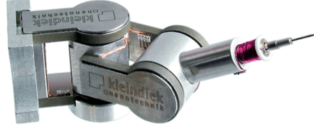
Figure 5.2: Micromanipulator used for mechanical actuation of auxetic metasurfaces of nanoscale thickness. The micromanipulator tip applies a force to the metasurface through piezoelectric actuators [157].
