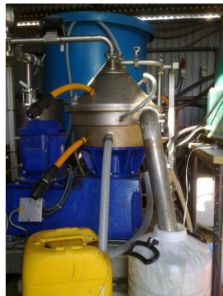
Figure 10.- Continuous centrifuge Alfa Laval Clara 15. University of Almeria, Spain
