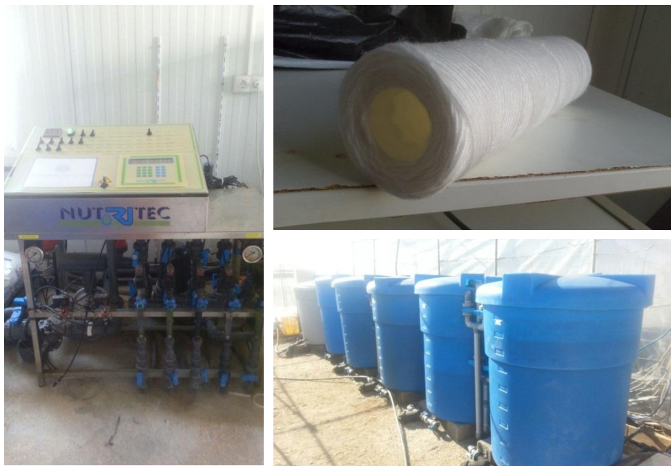
Figure 33.- Left: automatic irrigation and fertilization device (Nutritec N-9000) used for the preparation of fresh culture medium. Right: water filter cartridge used to eliminate solid particles before fresh medium addition to the raceway and tanks with nutrients solutions used by the automatic irrigation device to prepare the culture medium.
