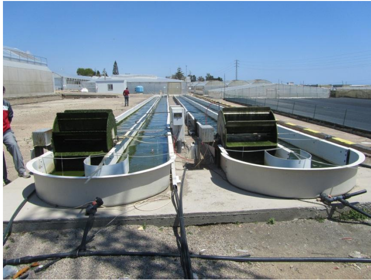
Figure 59.- Raceway reactors used simultaneously in this experiment. The setting-up of two reactors allowed pairs of experiments to be carried out under the same external conditions (wind, ambient temperature, solar radiation, etc.)
