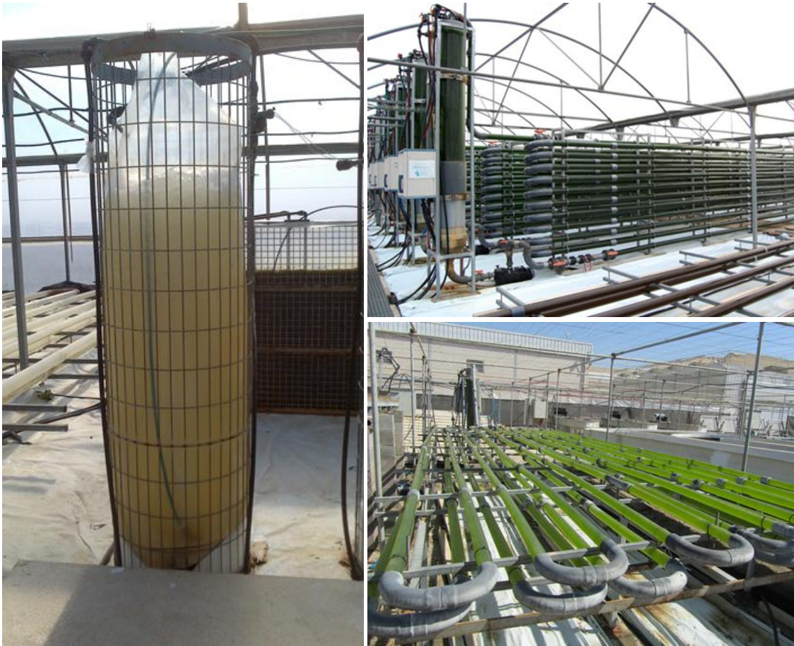
Figure 13.- Examples of closed systems for microalgae cultures (University of Almería, Spain). Left and right up: bubble bag column and vertical tubular photobioreactors. Right down: Horizontal tubular photobioreactor
