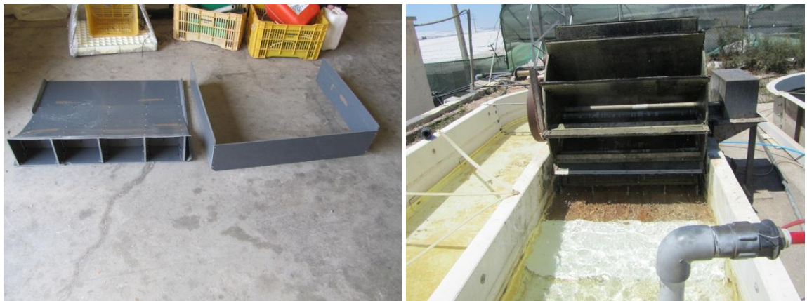
Figure 95.- Left: Shoe construction. Right: New 12 blades paddlewheel working with the shoe in position at the bed of the channel
