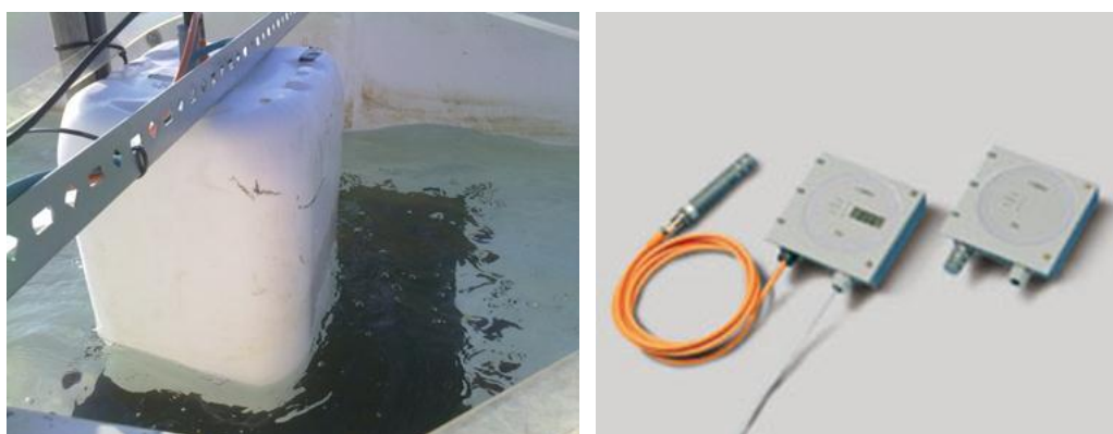
Figure 27.- Left: Detail of the fume hood which collected the gas reaching the surface for the measurement of its CO 2 concentration. Right: CO 2 probe located inside the fume hood and transmitter (picture obtained from www.vaisala.com )
