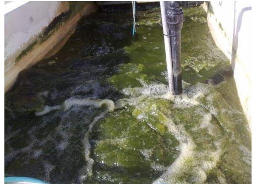
Figure 32.- Flue gas supply to the raceway. Left: flue gas production system with diesel boiler (white), gas compressor (black) and gas pressure vessel (blue). Right: sump view with flue gas bubbling in a microalgae culture.
