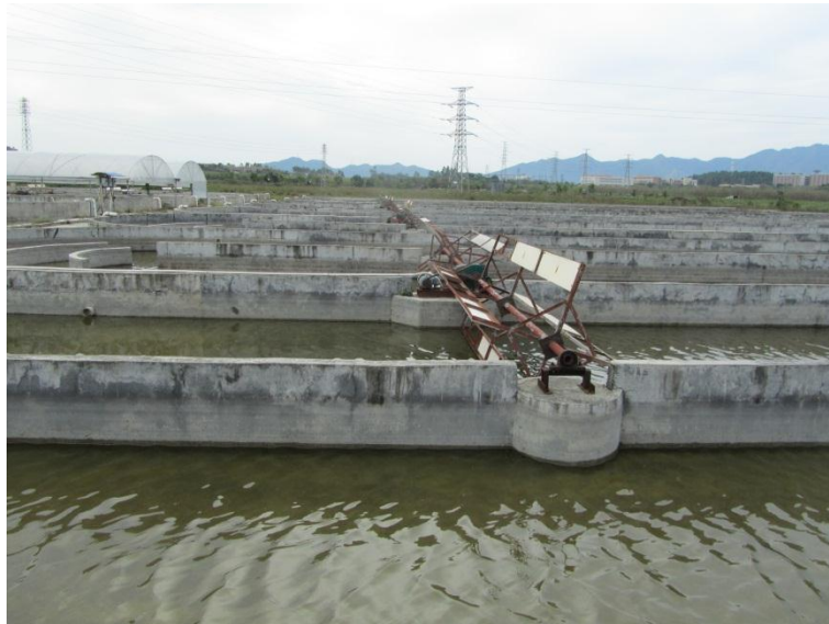
Figure 19.- Paddlewheel for fluid circulation and mixing (Foshan Innovation & Incubation Center of Renewable Energy Technology. Guangzhou Institute of Energy Conversion, China)
