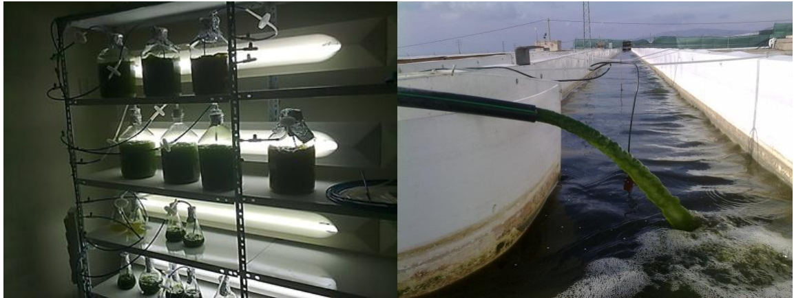
Figure 34.- Left: Flasks with different microalgae strains in the inoculum room. It is possible to see the illumination structure with fluorescent tubes and the agitation system with means of air bubbling. Right: Inoculation of the 100 m 2 raceway with 3 m 3 of microalgae culture obtained from the tubular reactors
