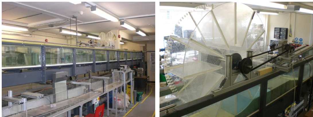
Figure 85.- Left: Flume. Right: Detail of paddlewheel, motor and shoe
