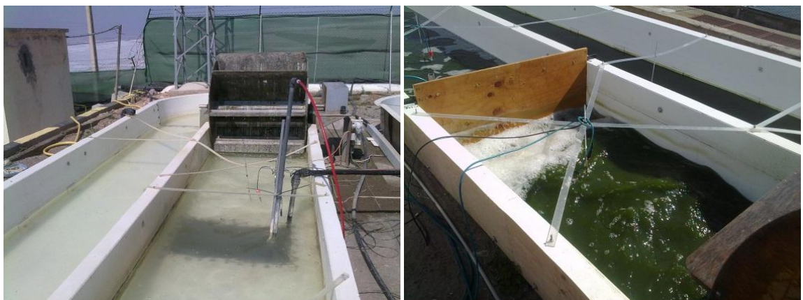
Figure 35.- Left: raceway before inoculation and without sump baffle. Right: raceway inoculated with Scenedesmus sp. with sump baffle in position
