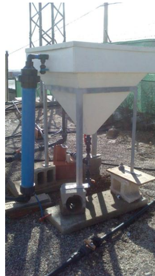
Figure 11.- Gravity sedimenter. Blue column is a mixing column where the culture broth is previously mixed with the flocculants.
