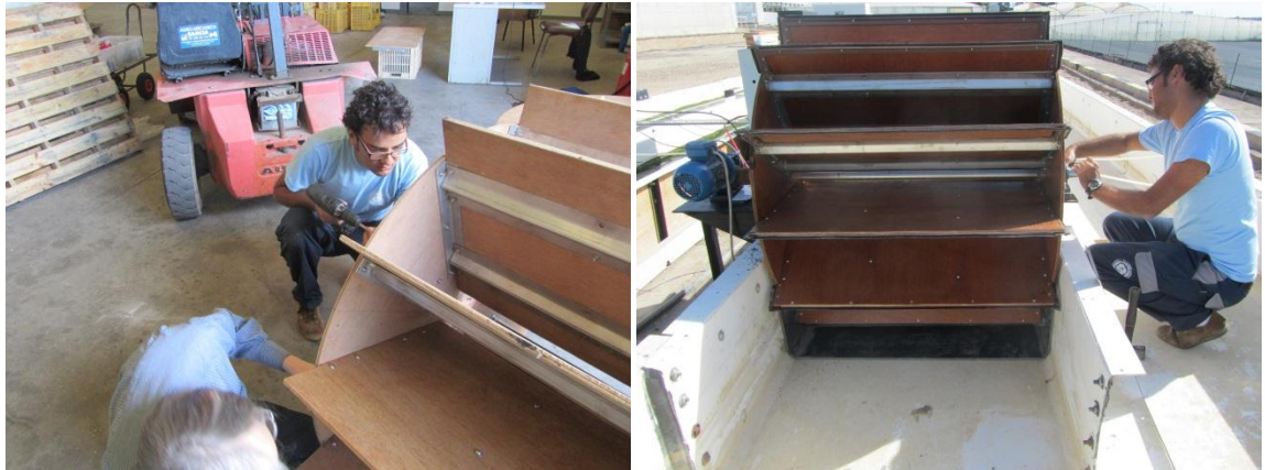
Figure 94.- Construction (left) and installation (right) of the new 12-blade paddlewheel
