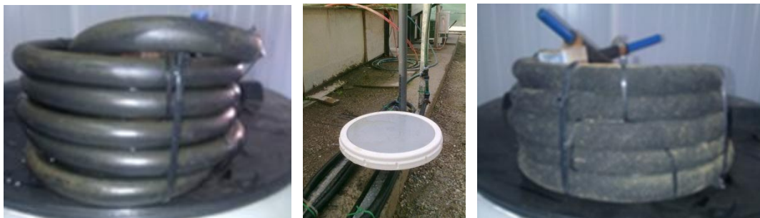
Figure 31.- Diffuser types used. From left to right: Membrane tube (type 1), membrane plate (type 2) and porous tube (type 3)
