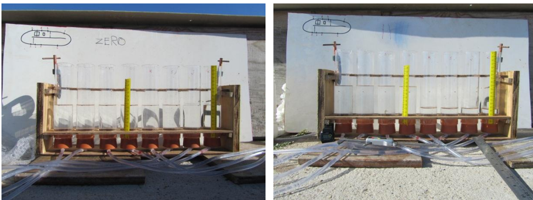
Figure 97.- Use of damping cylinders for measurement of head difference. Left: Zero position with the paddlewheel stopped and water level the same in all the damping cylinders. Right: Head difference in one of the experiments with the
