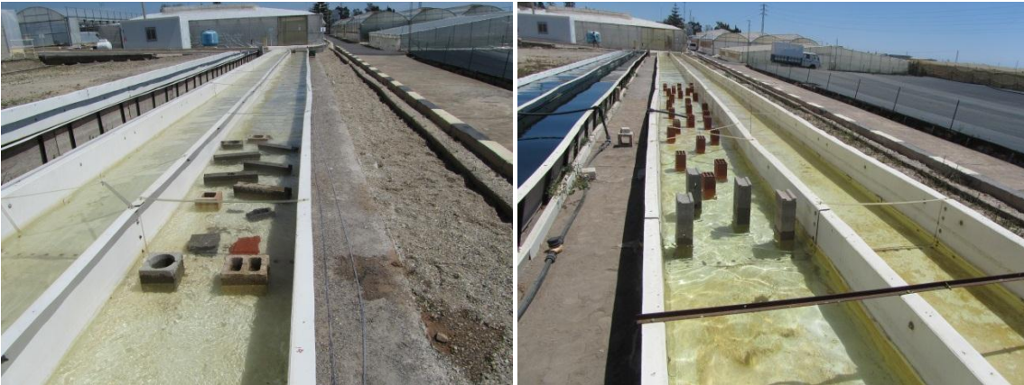
Figure 99.- Obstruction blocks used during the experiments to increase the head difference in the raceway. Left: Obstruction 1; Right: Obstruction 2
