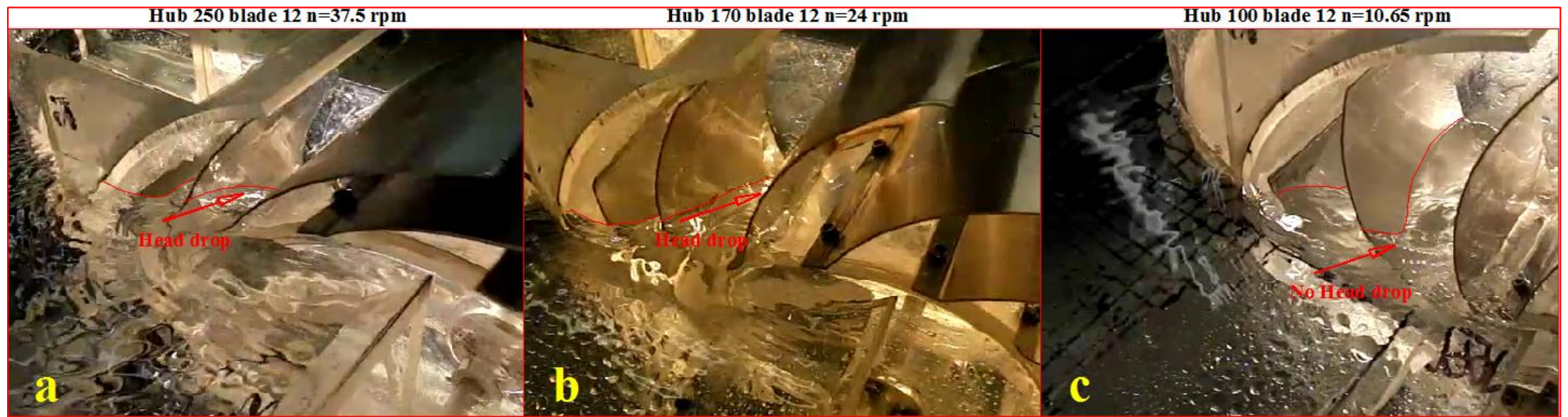
Figure 4.37: The inlet section for hub 250 mm, 170 mm, and 100 mm at max power output
