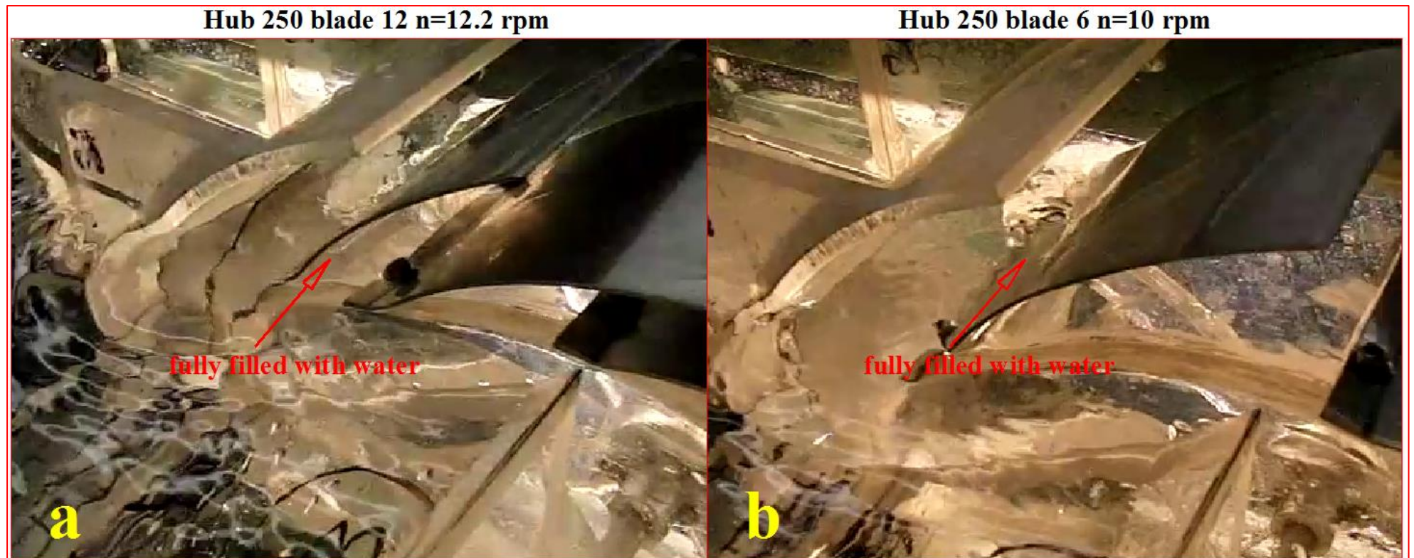
Figure 4.41: The inlet section for the 250 mm hub, 12 blade and 6 blade
