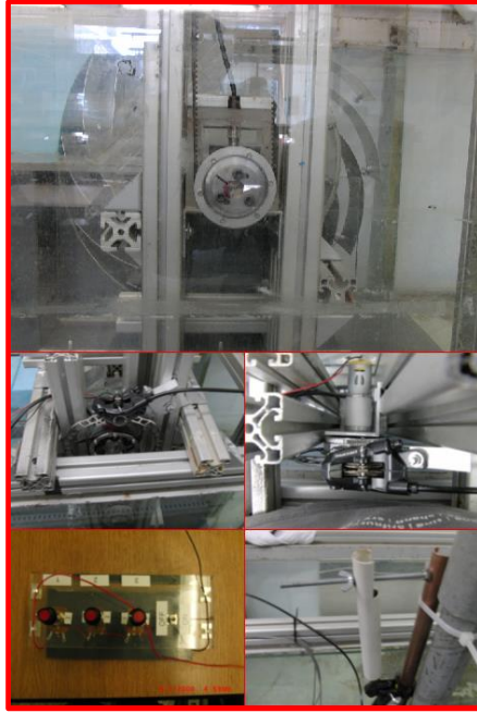
Figure 5.5: Depiction of the torquemeter, DC motor, disc brake and controoler of the load
